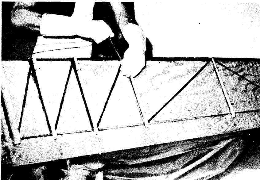
Figure 6. Winding the web and chord elements of TTG-3 on a removable wooden form.
