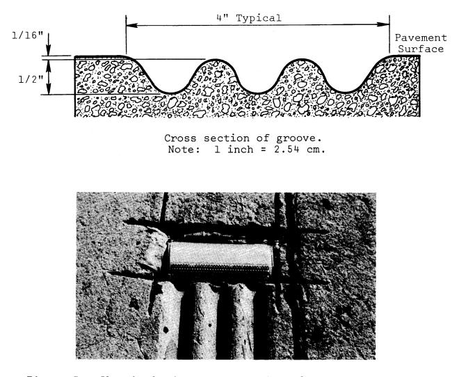
Figure 3. Sketch showing cross section of groove and marker emplaced in pavement.
