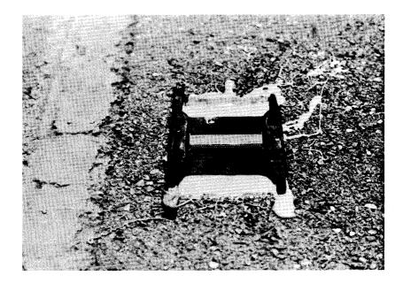
Figure 7. Casting and marker placed in groove.
