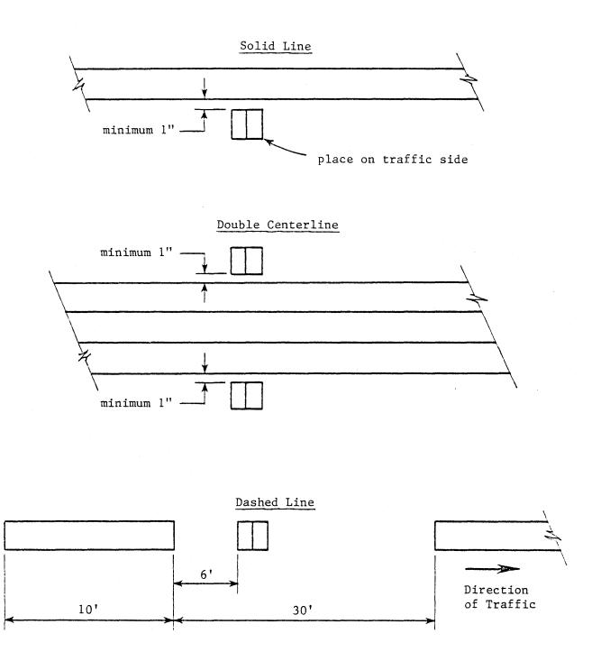
Figure 11. Placement of plowable raised pavement markers relative to centerlines and lane lines.
