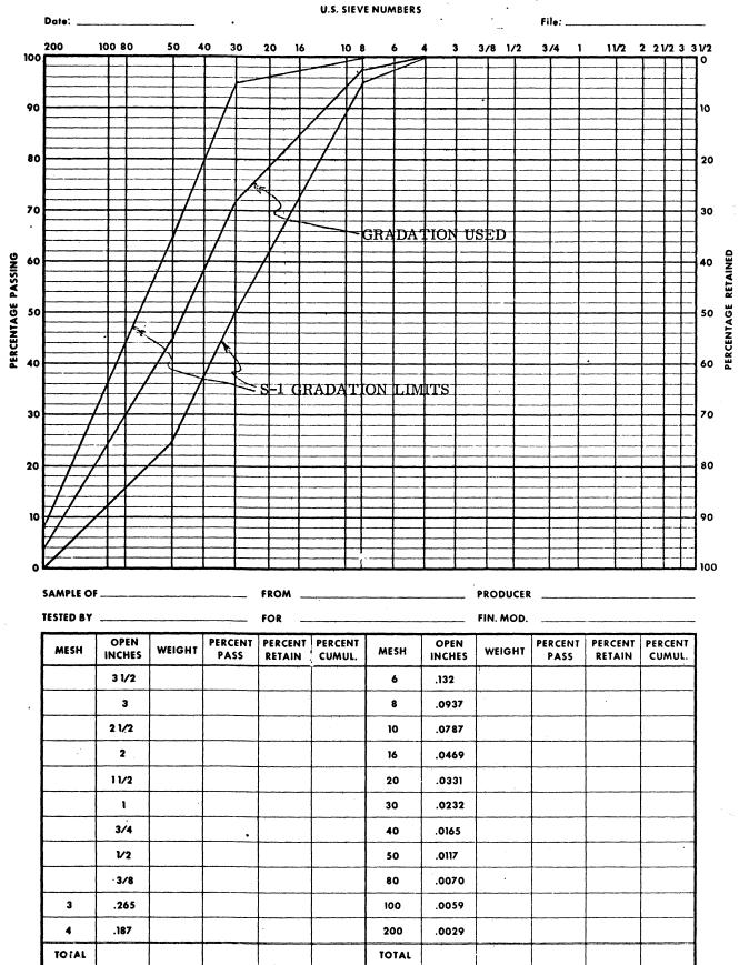
Figure A-1. Gradation used in S-1 Mix.
