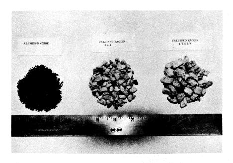
Figure 1. Sprinkle aggregate.
