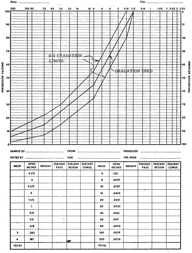
Figure A-2. Gradation used in S-5 Mix.
