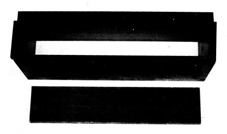
Figure 2. Test beam mold.
