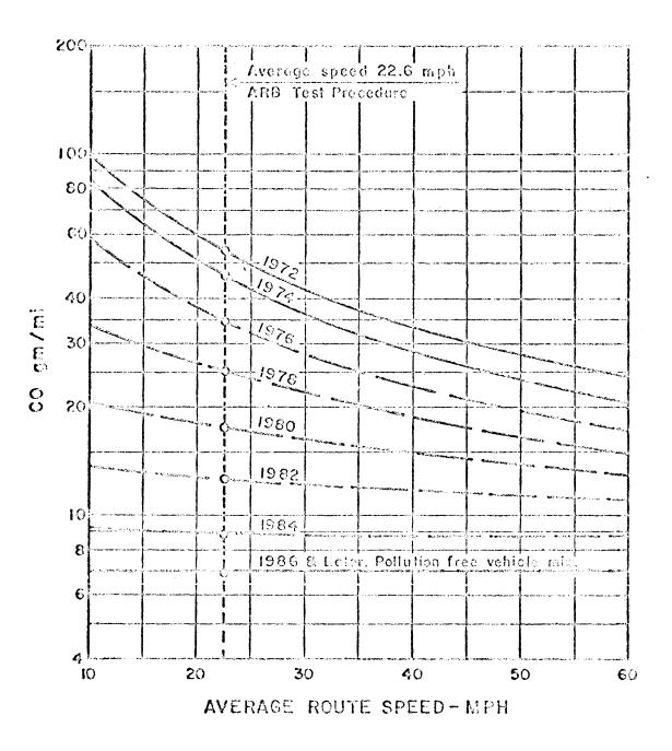
Figure 1: Emission factors for carbon monoxide vs. average route speed on freeways 10% HDV
