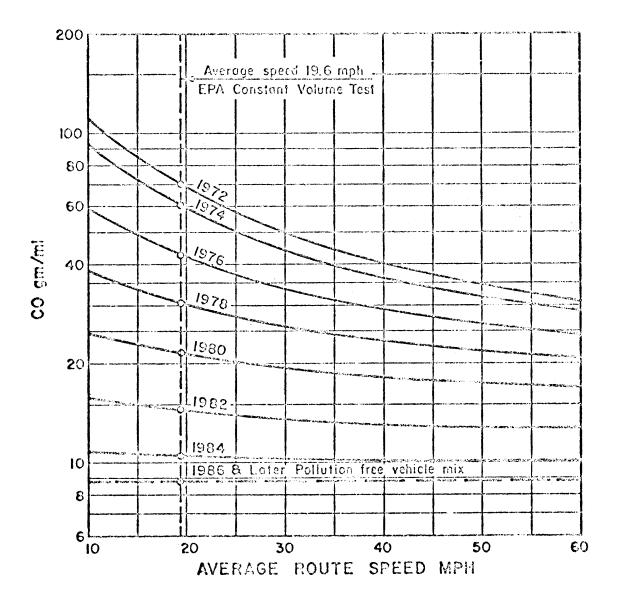
Figure 2: Emission factors for carbon monoxide vs. average route speed on city streets 10% HDV
