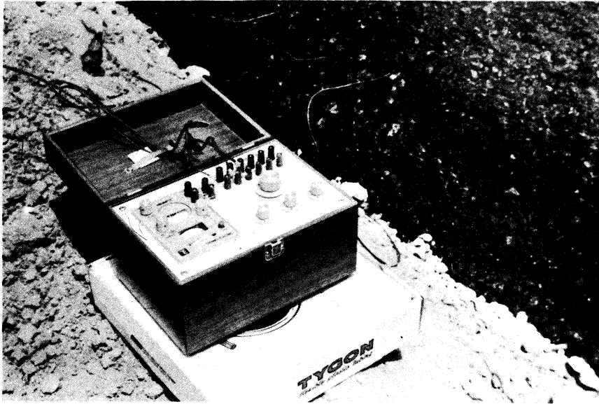
Figure 2. Null balance potentiometer and thermocouples used for taking temperature measurements.
