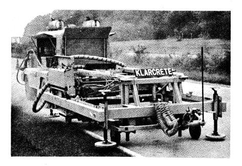
Figure 4. Full view of Klarcrete machine and compressor.
