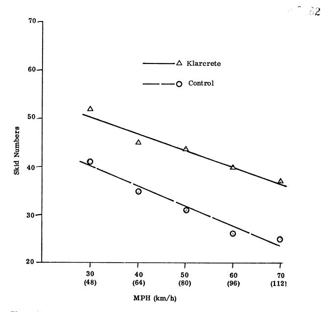
Figure 12. Skid test results for the traffic lane on the treated and untreated sections. Tests employed bald tire and a .020" water film thickness.
