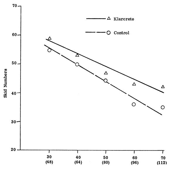
MPH (km/h) Figure 14. Skid test results for the traffic lane on the treated and untreated sections. New tire and a .040" water film thickness.
