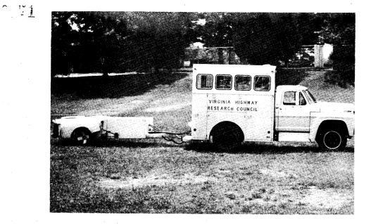
Figure 20. Research Council's skid-resistance measurement vehicle.
