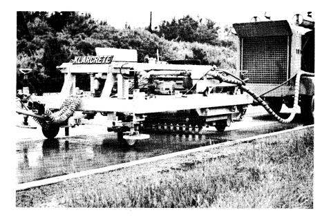
Figure 8. Klarcrete machine operating on wet pavement.
