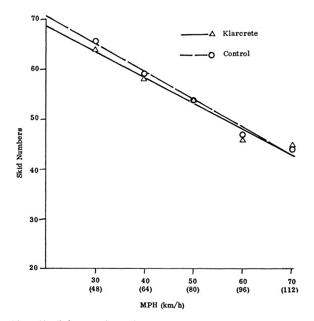
Figure 11. Skid test results for the passing lane on the treated and untreated sections. ASTM Method 274. .020" water film thickness.
