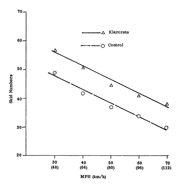
Figure 13. Skid test results for the passing lane on the treated and untreated sections. Tests employed bald tire and a .020" water film thickness.
