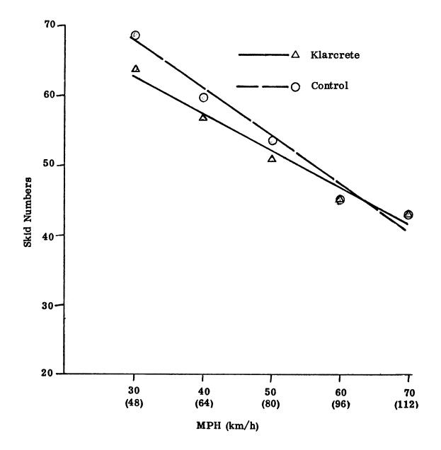
Figure 15. Skid test results for the passing lane on the treated and untreated sections. New tire and a .040" water film thickness.
