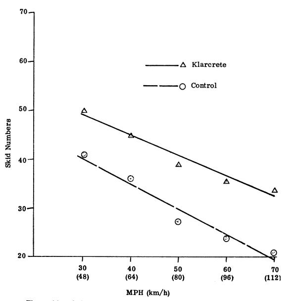
Figure 16. Skid test results for the traffic lane on the treated and untreated sections. Bald tire and a .040" water film thickness.
