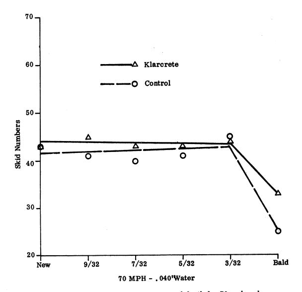
Figure 19. Skid results with respect to tire tread depth for 70 mph and .040" water film thickness for both control and Klarcrete passing lane sections.
