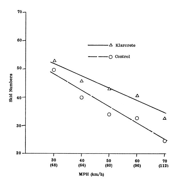
Figure 17. Skid test results for the passing lane on the treated and untreated sections. Bald tire and a .040" water film thickness.
