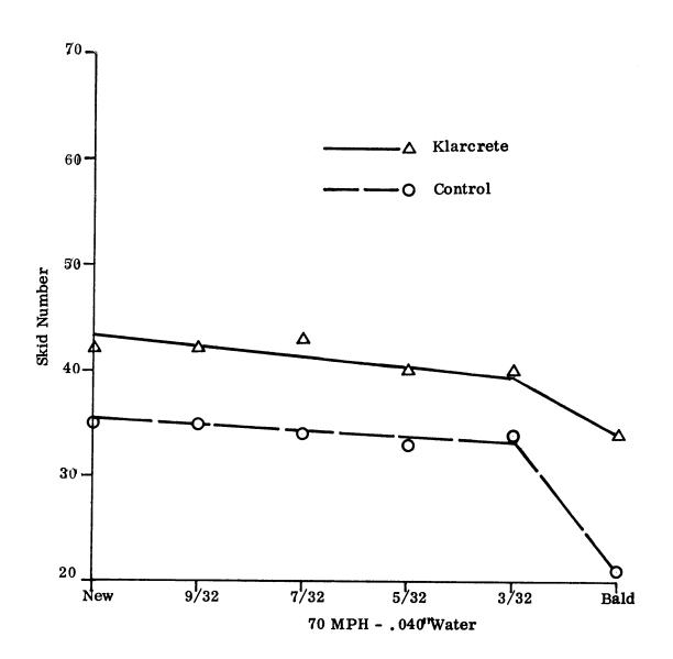
Figure 18. Skid results with respect to tire tread depth for 70 mph and .040" water film thickness for both control and Klarcrete traffic lane sections.
