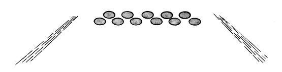
Figure 2. Arrangement of cutting heads for scabbler.
