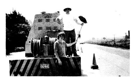
Figure 3. The 365 cfm, truck-mounted air compressor used in the evaluation.
