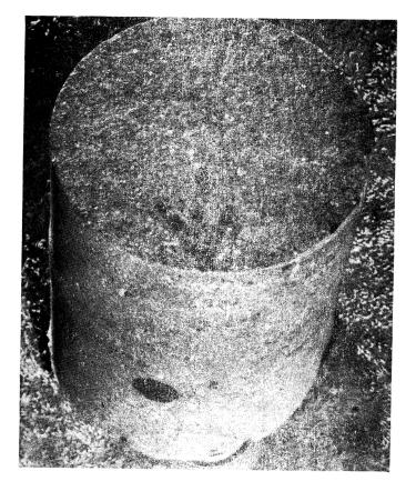
Figure 3. Longitudinal cracking in a concrete core with latex mortar overlay. Arrow on top of core denotes direction of traffic.
