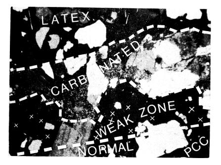
Figure 5. Thin section of bond area of core 5-2 showing latex mortar, carbonated zone, zone of weakness below the carbonated zone and normal PCC. The small x's indicate irregularly shaped voids. (50x, crossed polarizens.)
