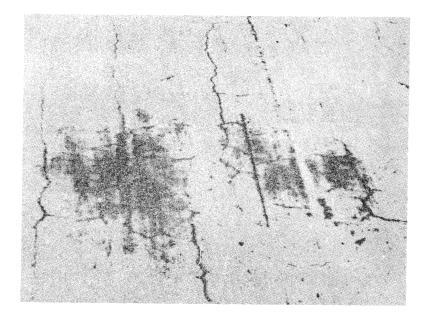
Figure 1. Typical cracking in the latex modified mortar overlay. Note that the deck is damp, which makes the cracks easily discernible.
