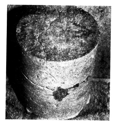
Figure 2. Transverse cracking in a concrete core with latex mortar overlay. Arrow on top of core denotes direction of traffic.
