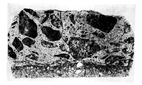
Figure 4. Section of core showing transverse cracking in the latex mortar overlay and the original concrete. A horizontal crack just below the bond line can be detected in the photograph.
