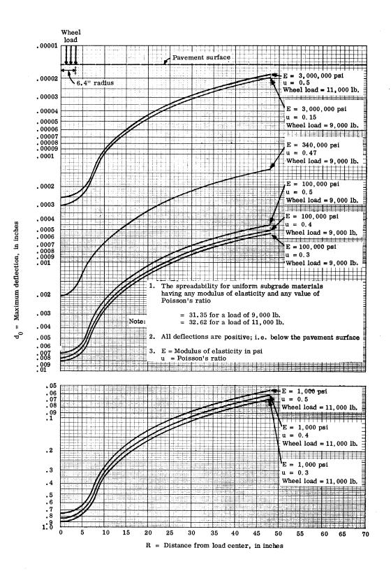
Figure 2. Deflection basin for a single layer with variable load, modulus of elasticity and Poisson's ratio.
