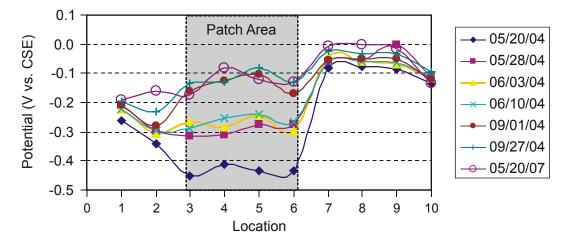
Figure 22. Column P12 Cu/CuSO<sub>4</sub> (CSE) Half-Cell Results: Route 29/Route 250 Over Route 654.
