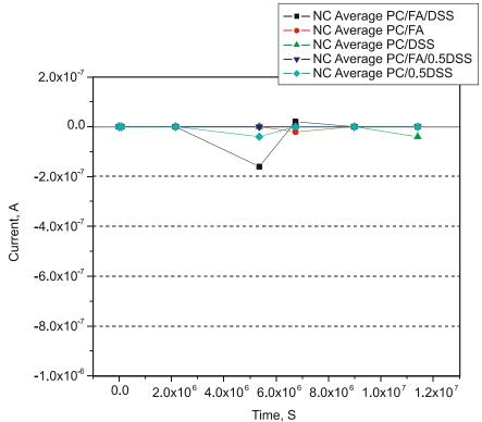
Figure 15. Average Corrosion Activity During Outdoor Exposure Based on Macrocell Measurements in Uncracked Specimens
