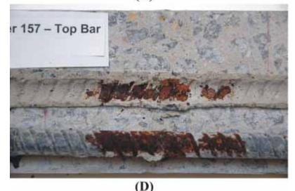
(D) Figure 20. (A) Top bar from specimen No. 157 showing corrosion centered at crack. (B) Underside of top bar showing significant corrosion on bottom side of rebar. Approximately 28% of top bar showing corrosion. (C) Two lower bars showing no signs of corrosion. (D) Close-up photograph of crack. (Mix PC/FA).
