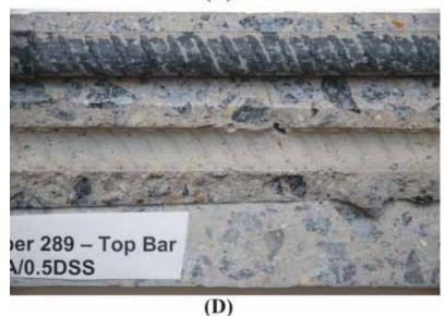
Figure 23. (A) Top bar from specimen No. 289 showing no corrosion at crack. (B) Underside of top bar showing no corrosion on bottom side of rebar. (C) Two lower bars showing no sign of corrosion. (D) Close-up photograph of crack. (Mix PC/FA/0.5DSS).
