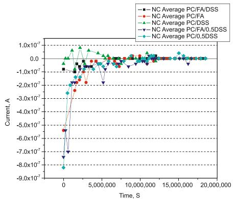
Figure 14. Average Corrosion Activity During Laboratory Exposure Based on Macrocell Measurements in Uncracked Specimens
