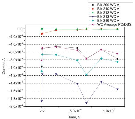
Figure 9. PC/DSS Cracked Specimens Demonstrated Increased Corrosion Activity During Outside Exposure Based on Macrocell Measurements
