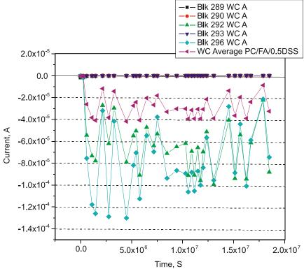
Figure 10. PC/FA/0.5DSS Cracked Specimens Demonstrated Intermediate Good Corrosion Resistance During Laboratory Exposure Based on Macrocell Measurements
