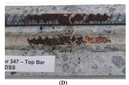
Figure 25. (A) Top bar from specimen No. 347 showing corrosion centered at crack. (B) Underside of top bar showing corrosion on bottom side of rebar. Approximately 34% of top bar showing corrosion. (C) Two lower bars showing no sign of corrosion. (D) Close-up photograph of crack. (Mix PC/0.5DSS).
