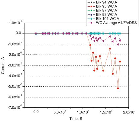
Figure 4. PC/FA/DSS Cracked Specimens Demonstrated Fairly Good Corrosion Resistance During Laboratory Exposure Based on Macrocell Measurements
