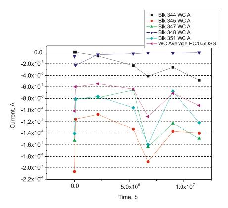
Figure 13. PC/0.5DSS Cracked Specimens Demonstrated Increase in Corrosion Activity During Outside Exposure Based on Macrocell Measurements
