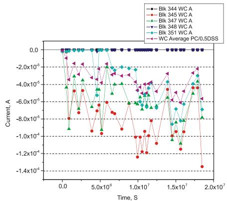
Figure 12. PC/0.5DSS Cracked Specimens Demonstrated Intermediate Good Corrosion Resistance During Laboratory Exposure Based on Macrocell Measurements
