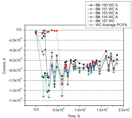
Figure 6. PC/FA Cracked Specimens Demonstrated Worst Corrosion Resistance During Laboratory Exposure
