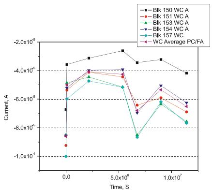
Figure 7. PC/FA Cracked Specimens Displayed Corrosion Activity During Outside Exposure Based on Macrocell Measurements
