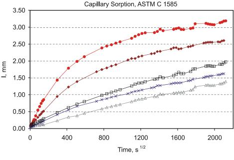
→ A4/FA → A4/DSS → A4/FA/0.5DSS → A4/0.5DSS → A4/FA/DSS Figure 3. Absorption Rate of Concretes (ASTM C 1585)
