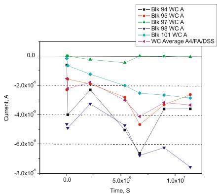
Figure 5. PC/FA/DSS Cracked Specimens Demonstrated an Increase in Corrosion Activity During Outside Exposure Based on Macrocell Measurements
