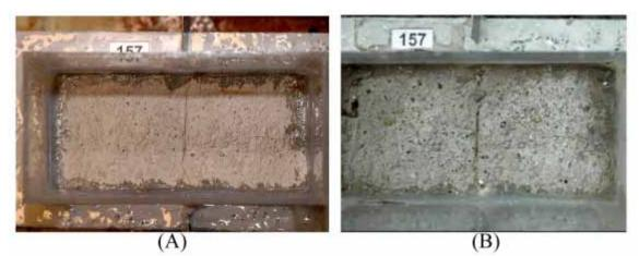
Figure 16. Typical view of specimen (A) before testing and (B) after testing, showing no outward signs of corrosion.
