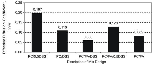
Figure 27. Effective Diffusion Coefficient for Different Mix Designs Based on Acid-Soluble Chloride Concentration Above Reinforcing Steel
