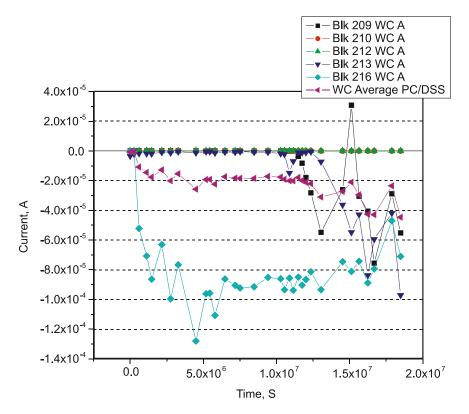
Figure 8. PC/DSS Cracked Specimens Demonstrated Intermediate Good Corrosion Resistance During Laboratory Exposure Based on Macrocell Measurements
