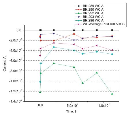
Figure 11. PC/FA/0.5DSS Cracked Specimens Demonstrated Increase in Corrosion Activity During Outside Exposure Based on Macrocell Measurements
