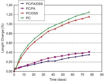
Figure 29. Length Change Due to Alkali-Silica Reactivity (ASTM C 1260)
