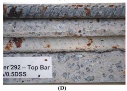
Figure 24. (A) Top bar from specimen No. 292 showing corrosion centered at crack. (B) Underside of top bar showing corrosion on bottom side of rebar. Approximately 19% of top bar showing corrosion. (C) Two lower bars showing no sign of corrosion. (D) Close-up photograph of crack. (Mix PC/FA/0.5DSS).
