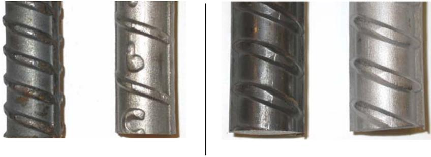
**Figure 2.** The surface appearance of 2101 duplex stainless steel (left) and MMFX-2 (right) in the as-received condition and with the mill scale removed by pickling in a hot nitric and hydrofluoric acid bath.
