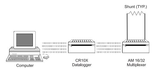
Figure 2. Schematic of Automated Test Setup
