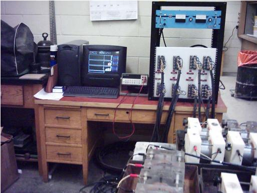
Figure 3. Automated RCPT Device
