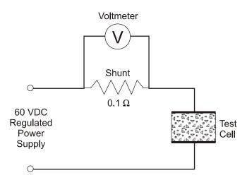
Figure 1. Basic RCPT Electric Circuit
