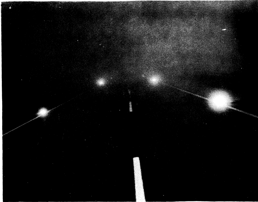
Figure 11. Runway lights spaced 120 feet apart in heavy fog.
