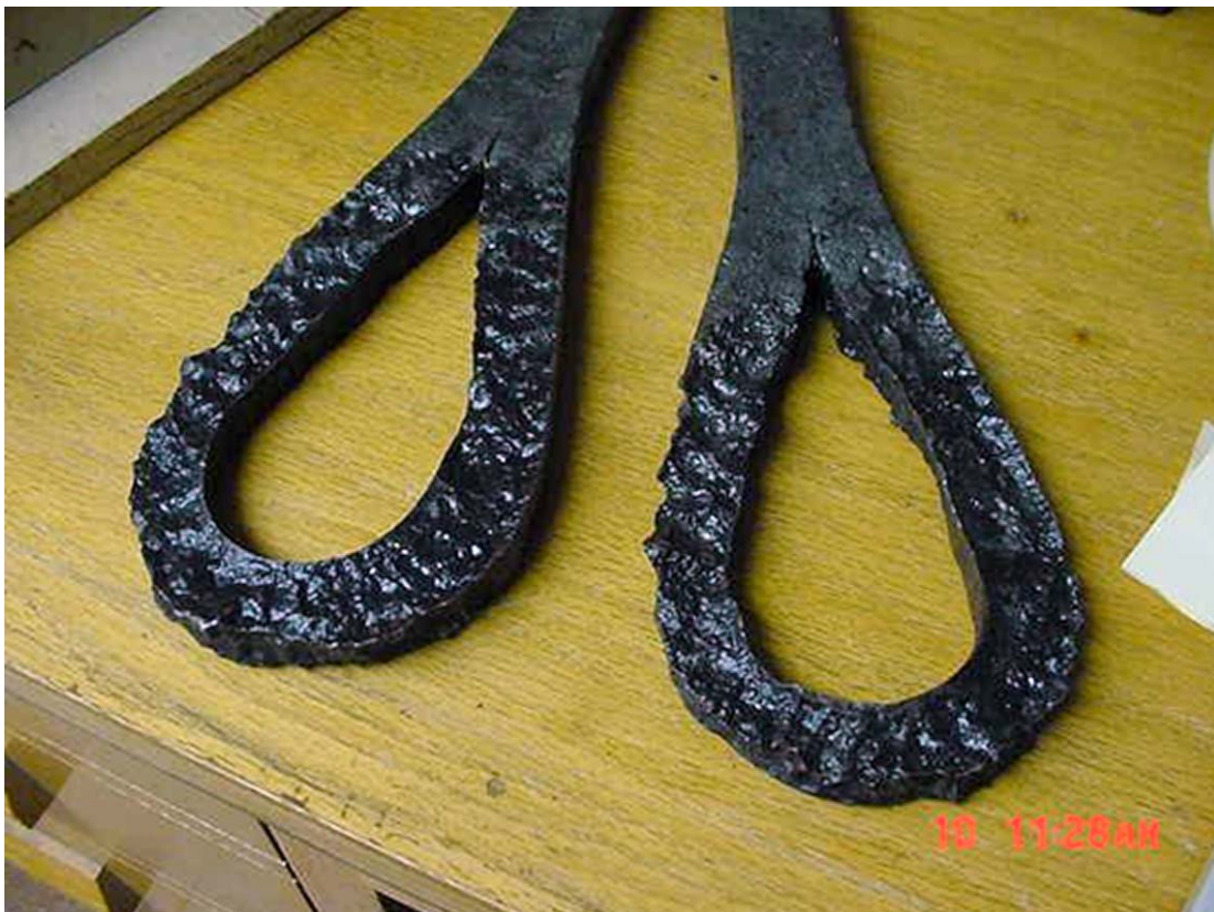
Figure 17. Typical Loop Bar Counters Showing Advanced Corrosion
