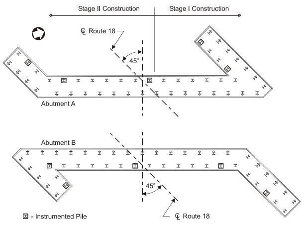
Figure 8. Layout of Foundation Piles
