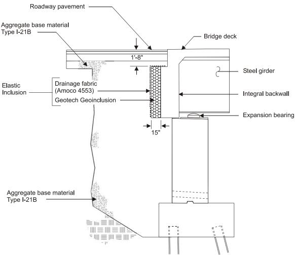
Figure 3. Cross Section of Abutment A
