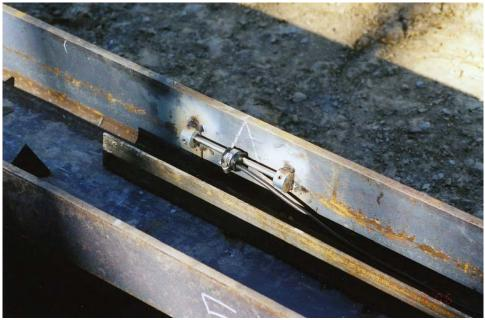
Figure 9. Strain Gage Welded To to Foundation Pile
