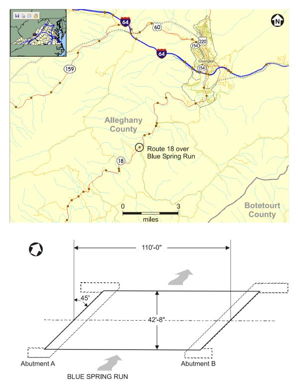
Figure 2. Site Location and New Bridge Layout
