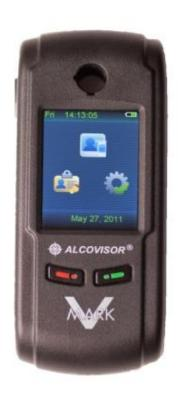
To turn off the Mark V, press and hold the green on/off button for 2 to 3 seconds. Note that the Mark V will automatically shut off after a few minutes if the unit is in the READY mode and no test has been performed.
