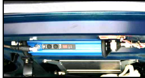
Figure 34. Pacific Crest radio unit.
