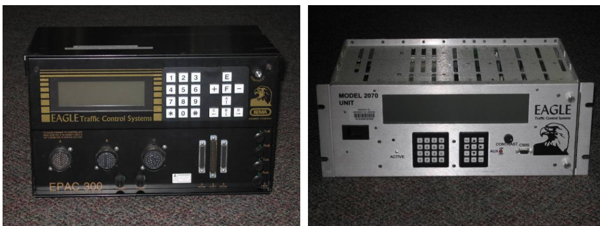
Figure 104. Eagle ECOM (left) and 2070 (right) controllers.
