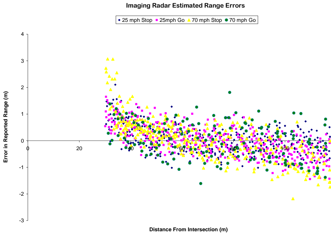
Figure 98. The difference between the range reported by the imaging radar and the “true” range as reported by the vehicle DAS plotted as a function of distance from the intersection. Each color/shape plots all five intersection approaches for the corresponding condition.
