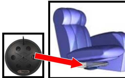
Figure 29. Vibrotactile transducers used in the rumble strip simulation.
