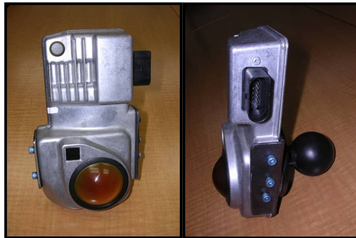
Figure 86. TRW Autocruise ACC radar front and side views with ball-mount attachment point used to place radar on signal mast arm and along the side of the roadway.
