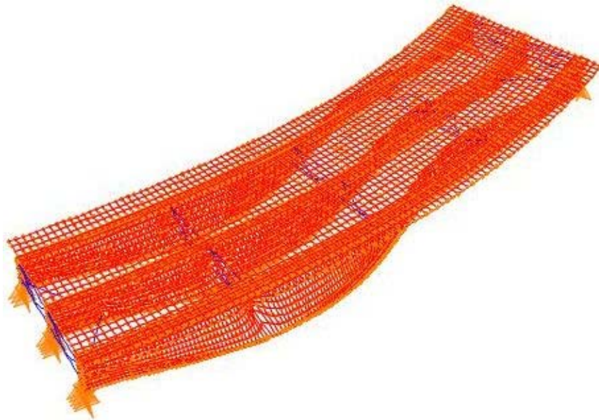
Figure 15d. Shell Model With Deck: Mode 4
