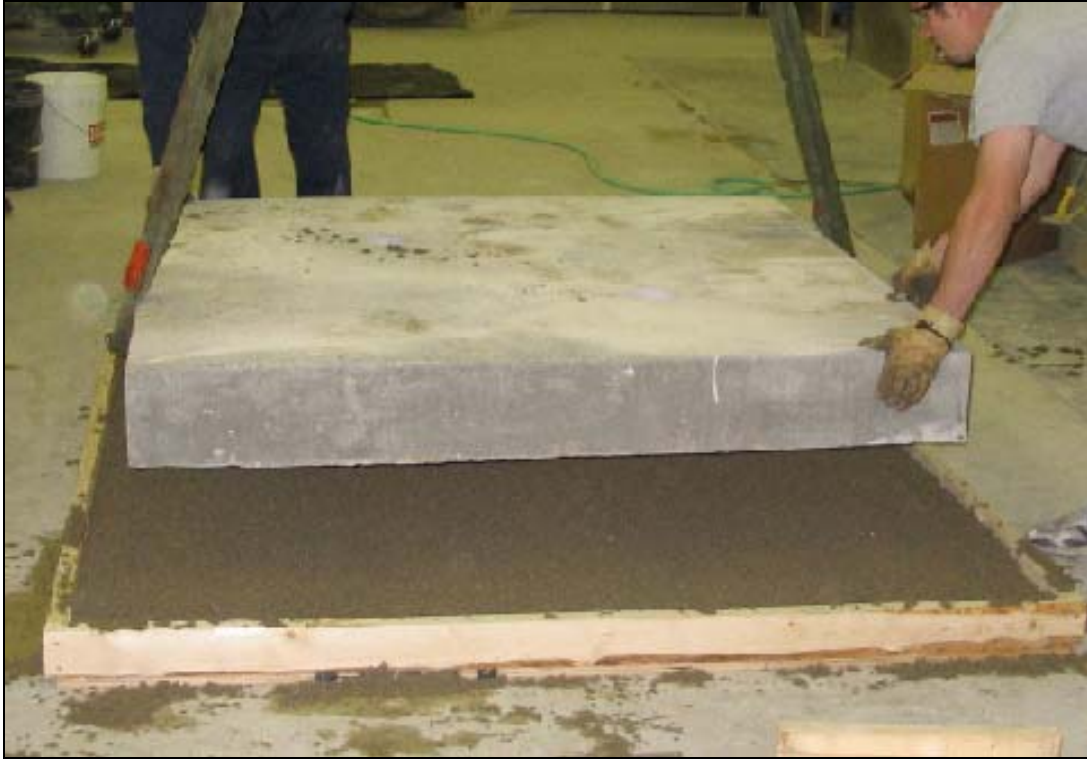
Figure 11: Transfer of the test slab onto the fresh mortar base in preparation for testing.
