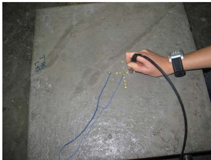
Figure 33: Testing configuration of sensors and point transducer on a concrete slab for surface wave velocity measurements.
