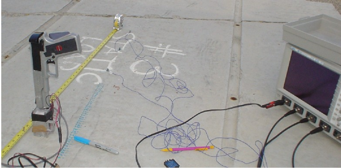
Figure 25: Experimental setup for the seismic reflection test.
