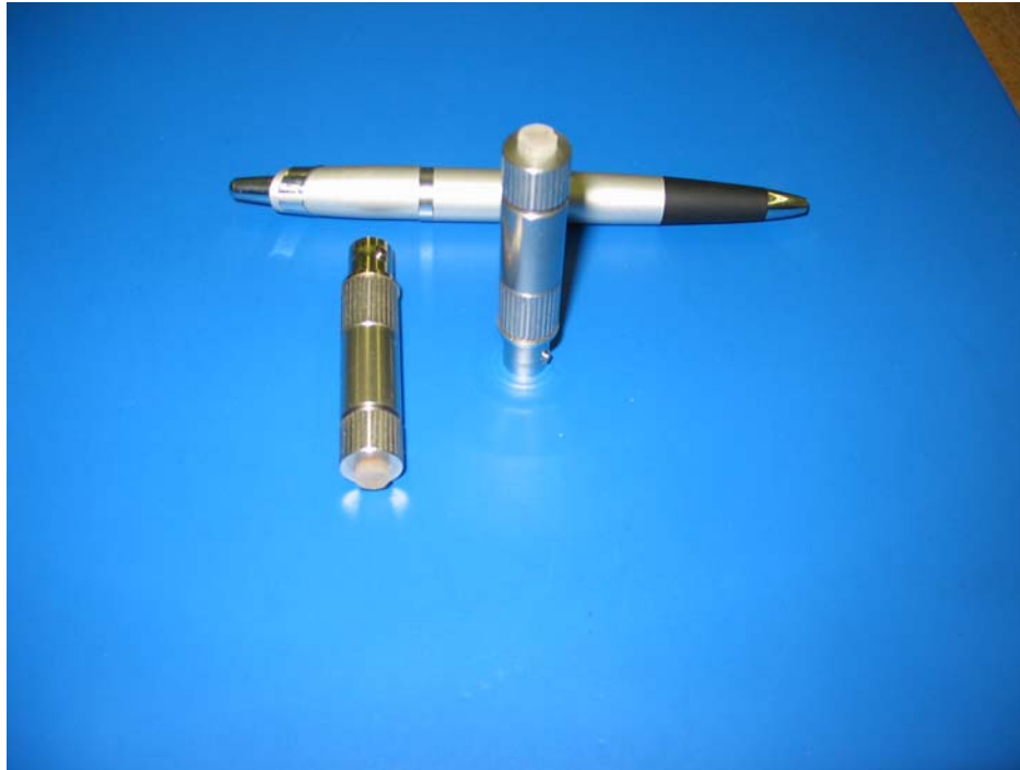
Figure 20: Dry-contact point transducers used for surface wave tests in concrete. Transducer center frequency is 200 kHz.
