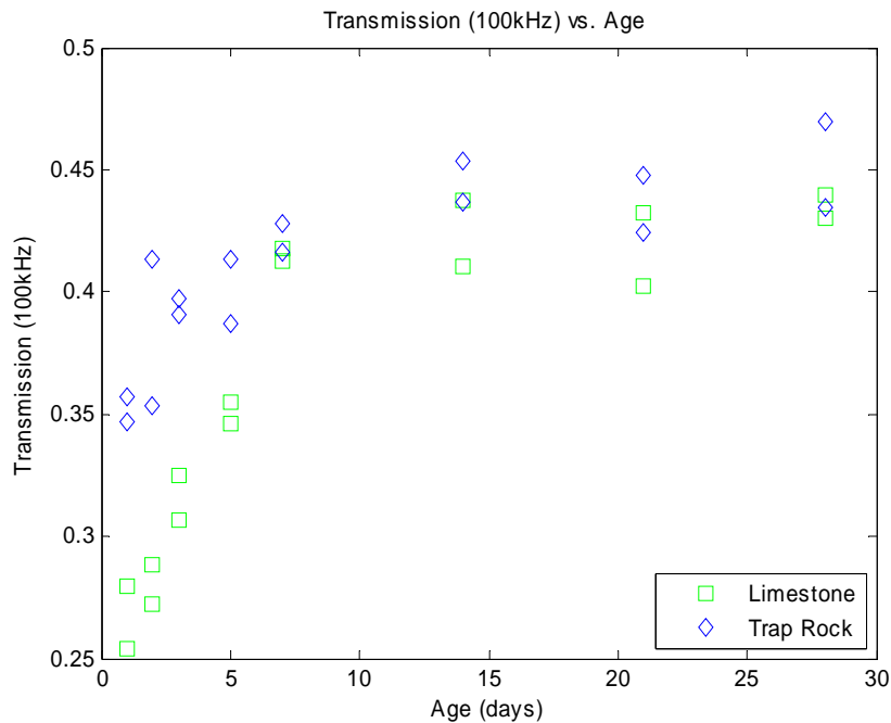
Figure 36: Transmission at 100 kHz as a function of age by aggregate type.
