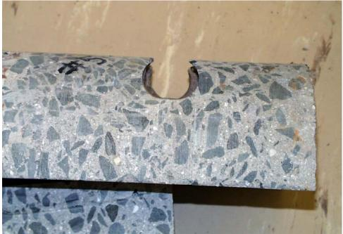
Figure 7. Core Through Faulted Transverse Joint and Wobbly Dowel Bar
