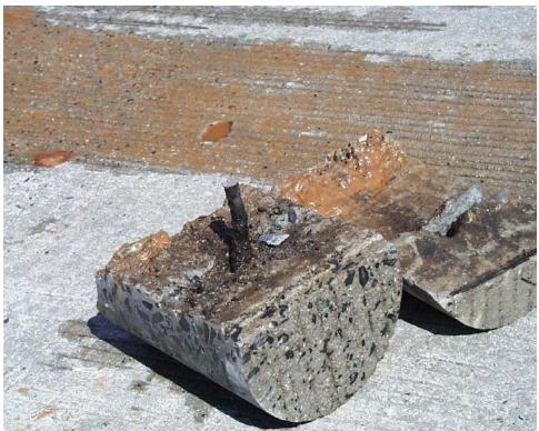
Figure 6. Core Through Faulted Longitudinal Joint and Bent Tie Rod
