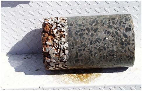
Figure 8. Clogged Drainage Layer
