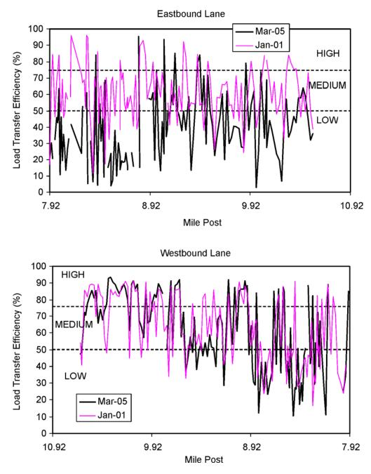
Figure 4. Load Transfer Efficiencies Measured with FWD test for 2001 and 2005
