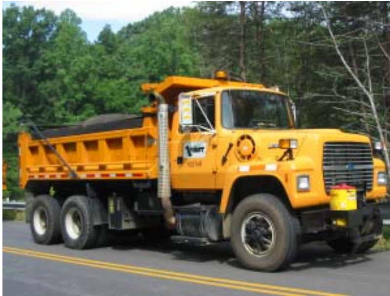
Figure 10 VDOT Dump Truck Used for Live Load Testing
