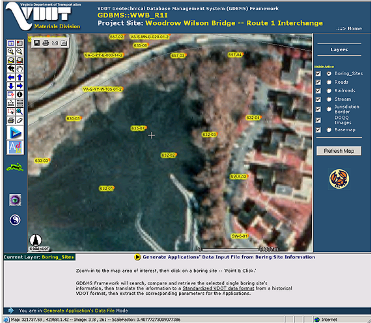
Figure 12. ADM Initialization and Borehole Selection Procedure for Generating Geotechnical Application Input Data File
