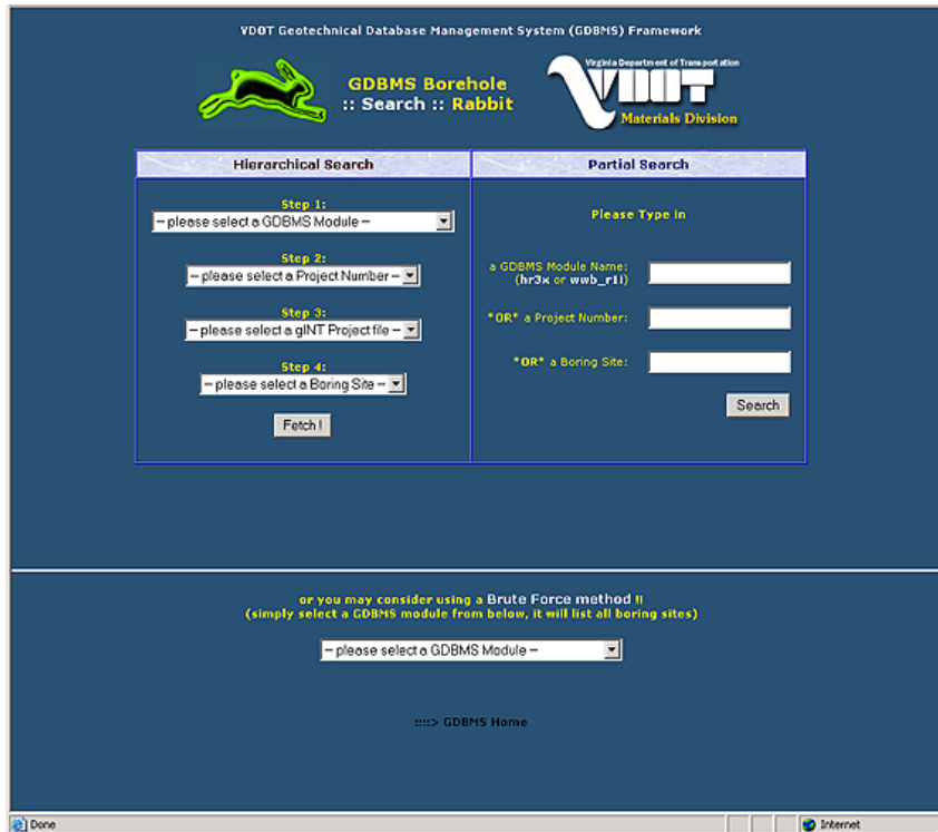
Figure 5. Main Borehole Data Search Interface - GDBMS Borehole Search Rabbit : Borehole data search interface provides three different search modes: (a) Hierarchical search mode to constrain the query to get an exact borehole data, (b) Partial search mode to create a “matching” query to all existing GDBMS data, and (c) Site module search mode for a full listing of borehole data.
