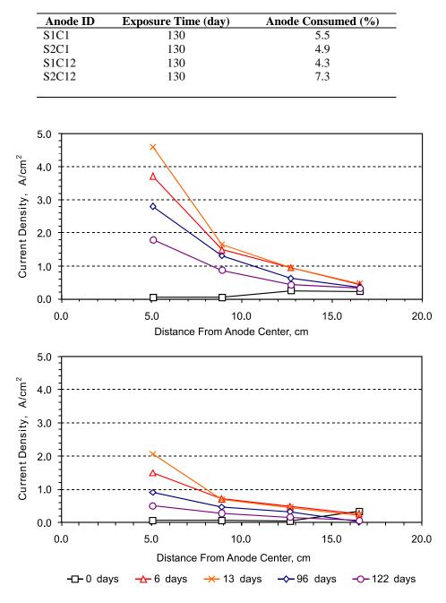
Figure 18. Current Density Measurements at Sacrificial Anode Monitoring Devices in (top) Pier 1 and (bottom) Pier 12
