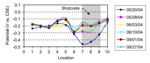
Figure 13. Half-Cell Measurements Versus Location for Column P1, Which Contains Sacrificial Anodes
