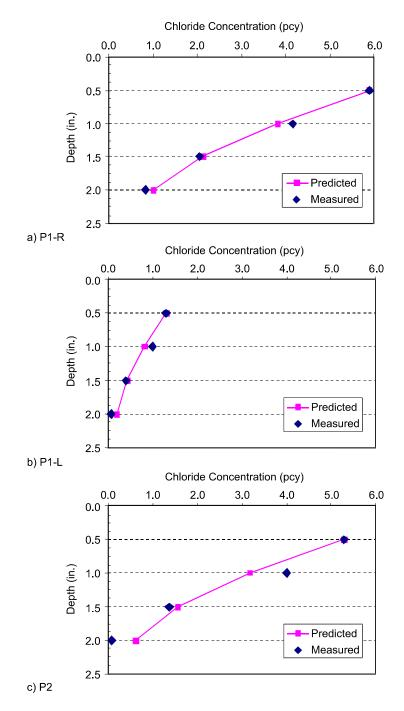
Figure 11. Chloride Concentration Profiles Adjacent to Repairs at Location P1-R, P1-L, and P2
