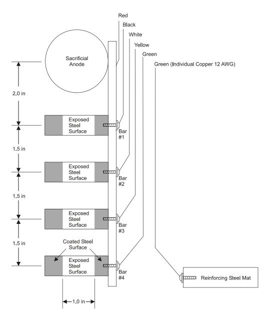
Figure 7. Sacrificial Anode Monitoring Device
