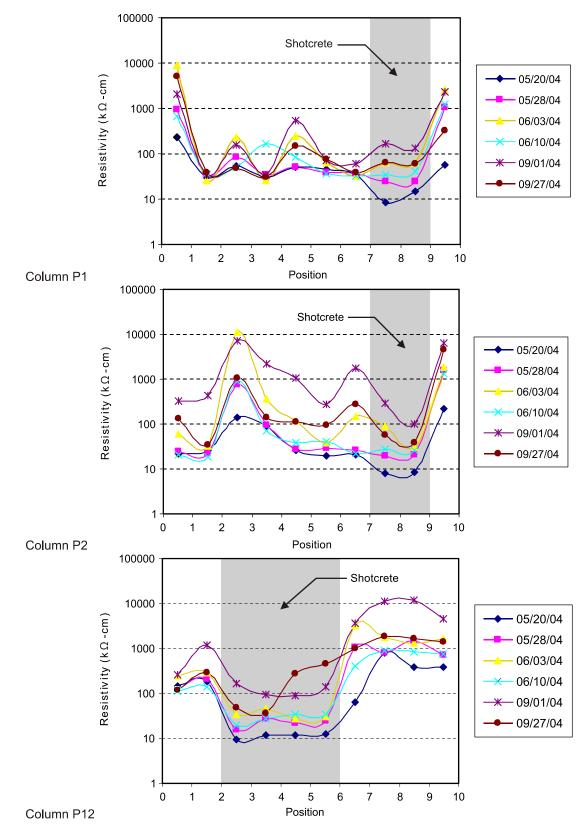
Figure 16. Post-repair Resistivity of Concrete Versus Location
