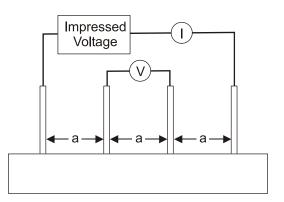
Figure 6. Four-Pin Resistivity Test Schematic
