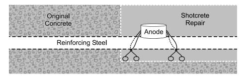
Figure 1. Diagram of Anode and Placement
