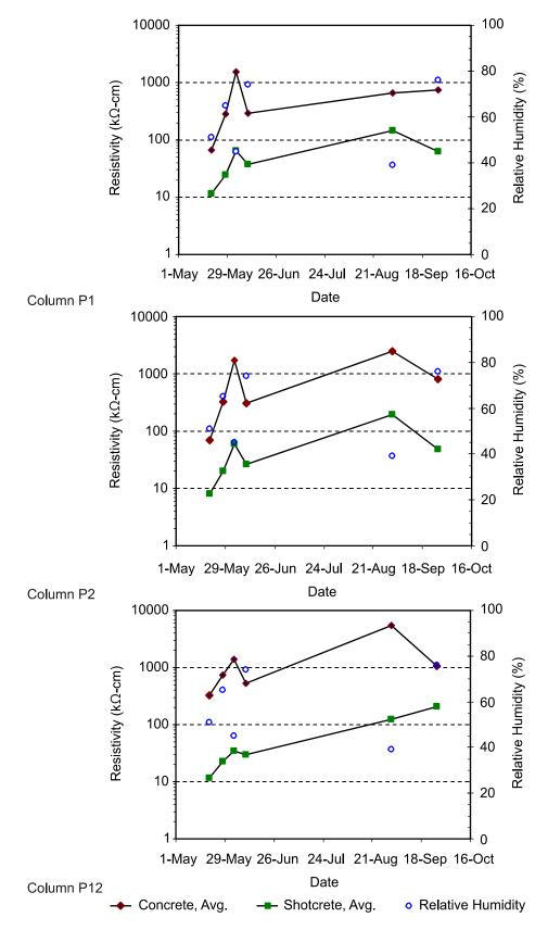
Figure 17. Post-repair Resistivity of Concrete Versus Time
