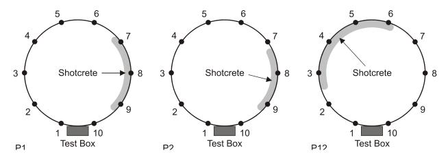
Figure 5. Electrical Test and Shotcrete Repair Locations on Each Column
