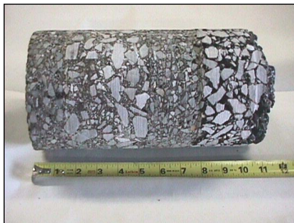
Figure 13. Typical HMA core extracted from Section H at the Virginia Smart Road.
