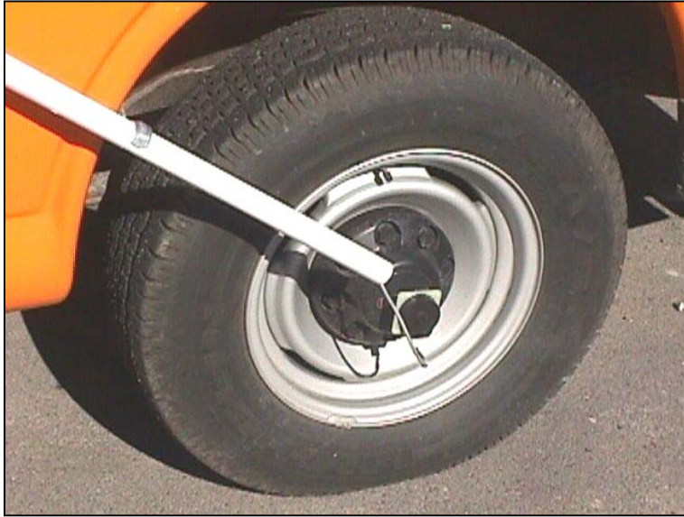
Figure B6. DMI mounted on GPR van wheel.
