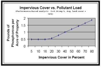
Figure 3.2 - Impervious Cover vs. Pollutant Load (from VA SWM Bulletin No. 4)
