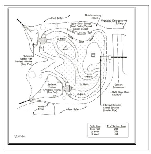
Figure 4.2 - Enhanced Extended Detention Basin
