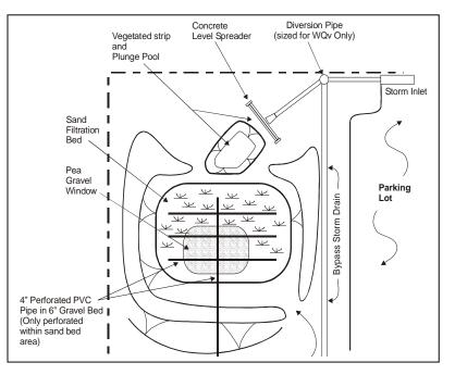
Figure 5-4 Pocket Sand Filter - Plan View (after Claytor and Schueler, 1996).
