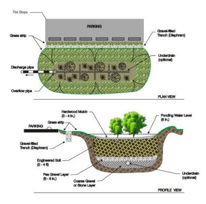
Figure 5.3 - Schematic Drawing of a Typical Bioretention Unit.
