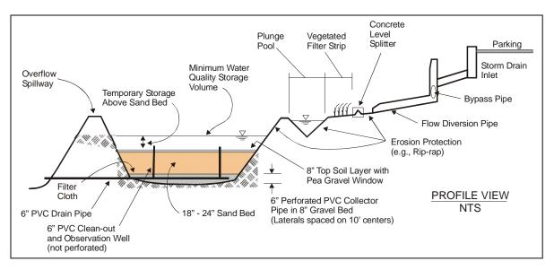
Figure 5-5. Pocket Sand Filter - Profile View (after Claytor and Schueler, 1996)
