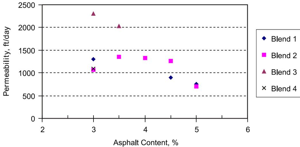
**Figure 3. Permeability Results for Laboratory Mixtures.**
