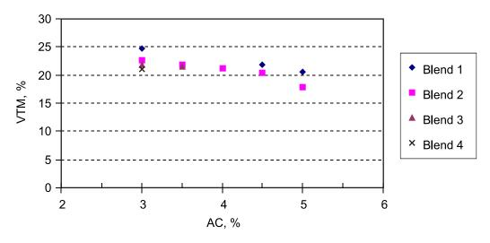
Figure 1. Voids of Gyratory Specimens.
