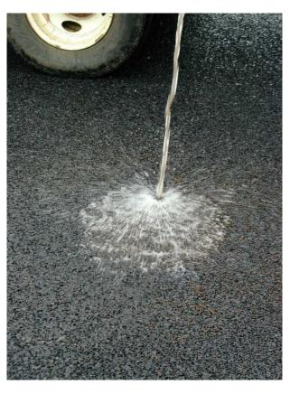
Figure 5. Water Draining Through Drainage Layer.
