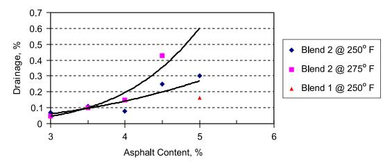
Figure 2. Asphalt Drainage Results for Laboratory Mixtures.
