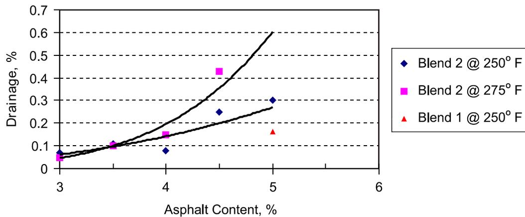
Figure 2. Asphalt Drainage Results for Laboratory Mixtures.
