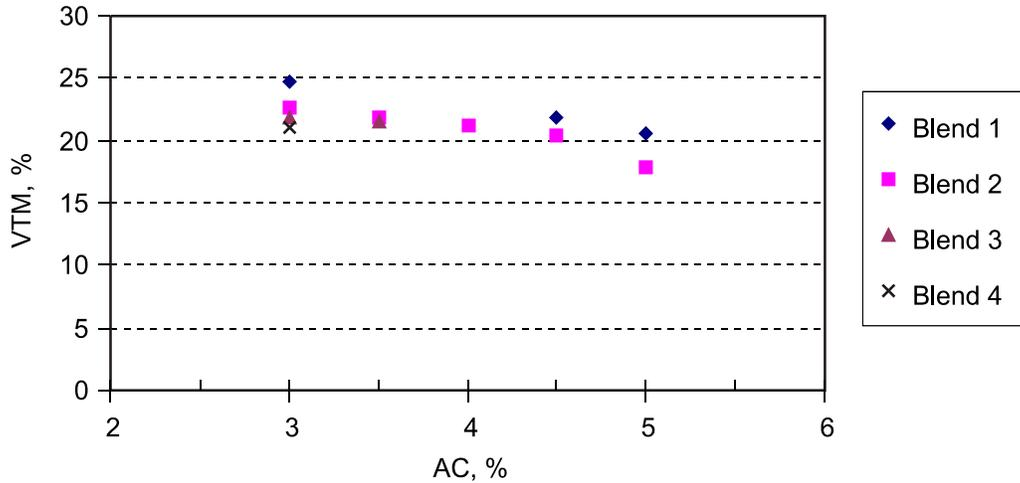
Figure 1. Voids of Gyratory Specimens.
