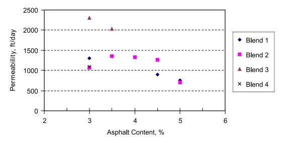
Figure 3. Permeability Results for Laboratory Mixtures.
