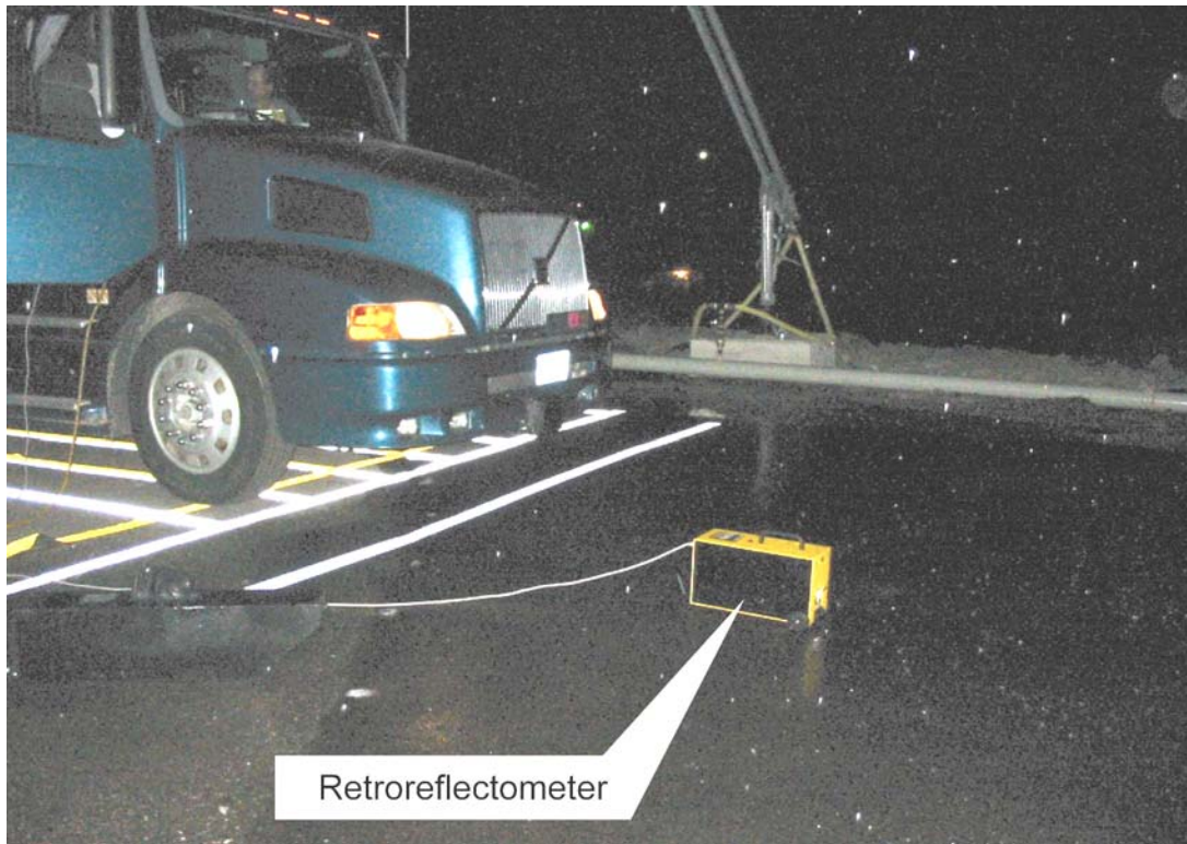
Figure 9. The alignment grid, the wet truck and the retroreflectometer in use at the experimental area.
