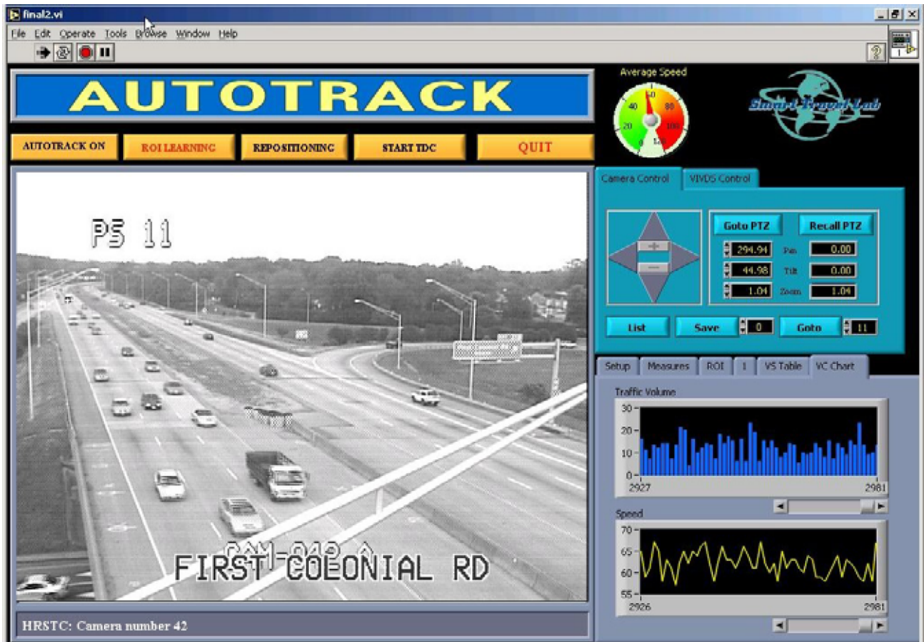
Figure 5. Phase II Autotrack User Interface
