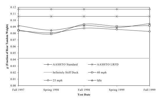
**Figure 15.** Summary of the design wheel load distribution factor, g. Values based on mid-span strain data.
