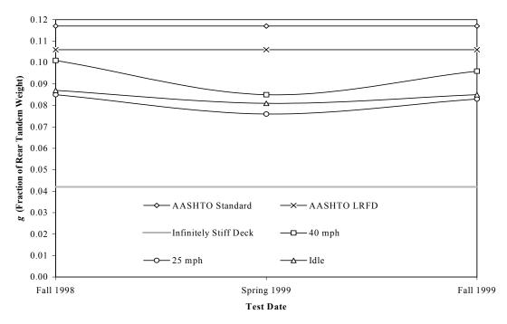
**Figure 16.** Summary of the design wheel load distribution factor, g. Values based on mid-span deflection data.
