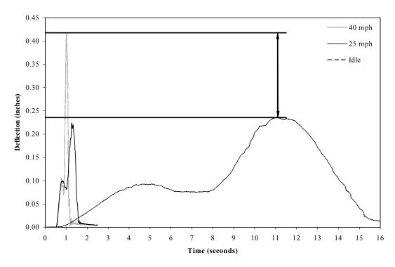
**Figure 10.** Typical Tom's Creek Bridge composite girder response (mid-span deflections) due to heavy truck loading.
