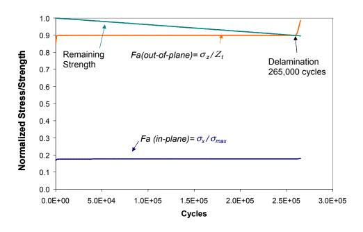
**Figure 19.** Graphical representation of remaining strength and the stress on the critical element. This analysis is shown for an applied moment, 85% of the ultimate moment capacity.
