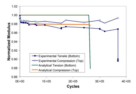
**Figure 18.** Stiffness reduction (predicted and measured) curve for the girder fatigued at 53% of the ultimate moment capacity.
