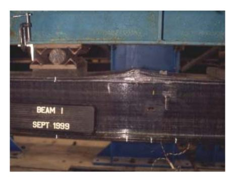
**Figure 8.** Failure of the compression flange for removed Tom's Creek Bridge FRP composite Girder 1. Note failure occurs at mid-span.
