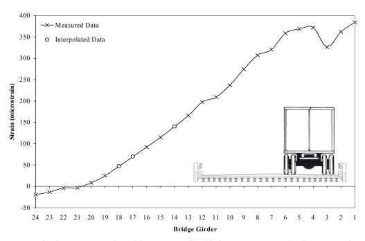
**Figure 13.** Typical Tom's Creek Bridge composite girder response under heavy truck crossing, right lane 40 mph.
