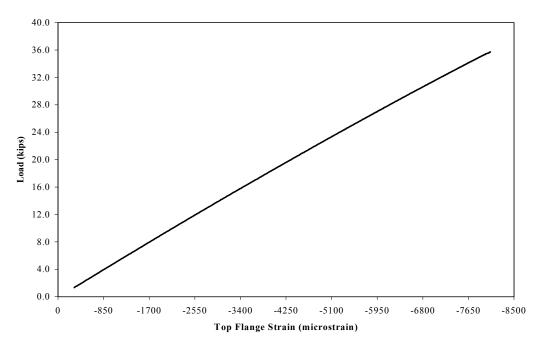
**Figure 17.** Load versus top flange strain to failure for FRP composite girder 2, failed after fifteen months of service in the Tom's Creek Bridge.
