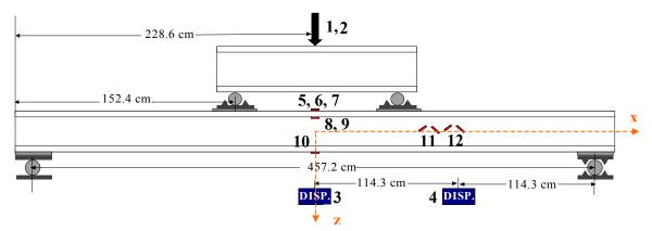
**Figure 6.** Schematic for the instrumentation used in the characterization of strength and fatigue. 1. Actuator Load, 2. Actuator deflection, 3. Mid-span Deflection, 4. Quarter Point Deflection, 5. Top Center Bending Strain, 6. Top Right Bending Strain, 7. Top Left Bending Strain, 8. Top Right Flange Bending Strain, 9. Top Left Flange Bending Strain, 10. Bottom Center Bending Strain, 11. Shear Strain 1 in outside of the constant moment region, 12. Torsional Strain at the ½ point.
