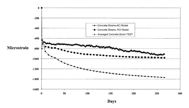
Figure 17: Variation of Concrete Strains vs. Time
