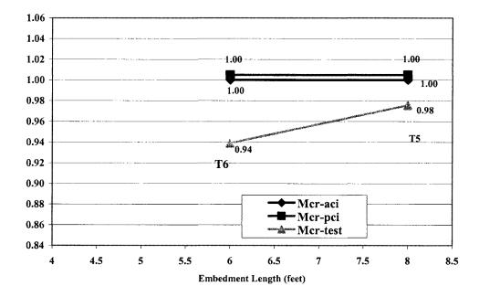
Figure 21: Ratio of Test and Theoretical Cracking Moments for the HPNWC Beams
