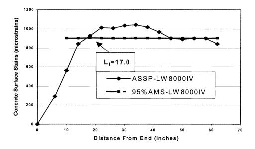
Figure 10: Averaged Strain Profile for Both HPLWC Type IV Test Beams
