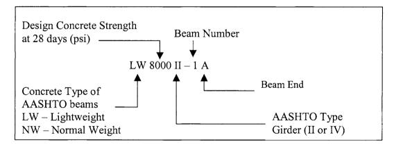
Figure 1: Test Beam Nomenclature
