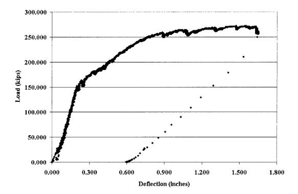
Figure 12: Load Deflection Curve: Beam LW8000II-2C-72
