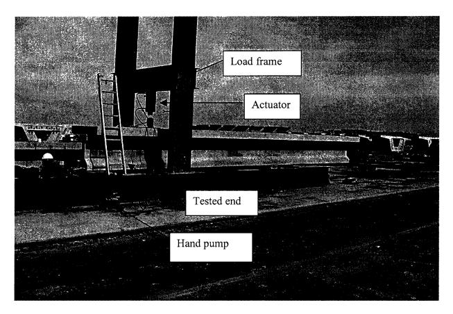
Figure 8: Load Frame and Test Setup
