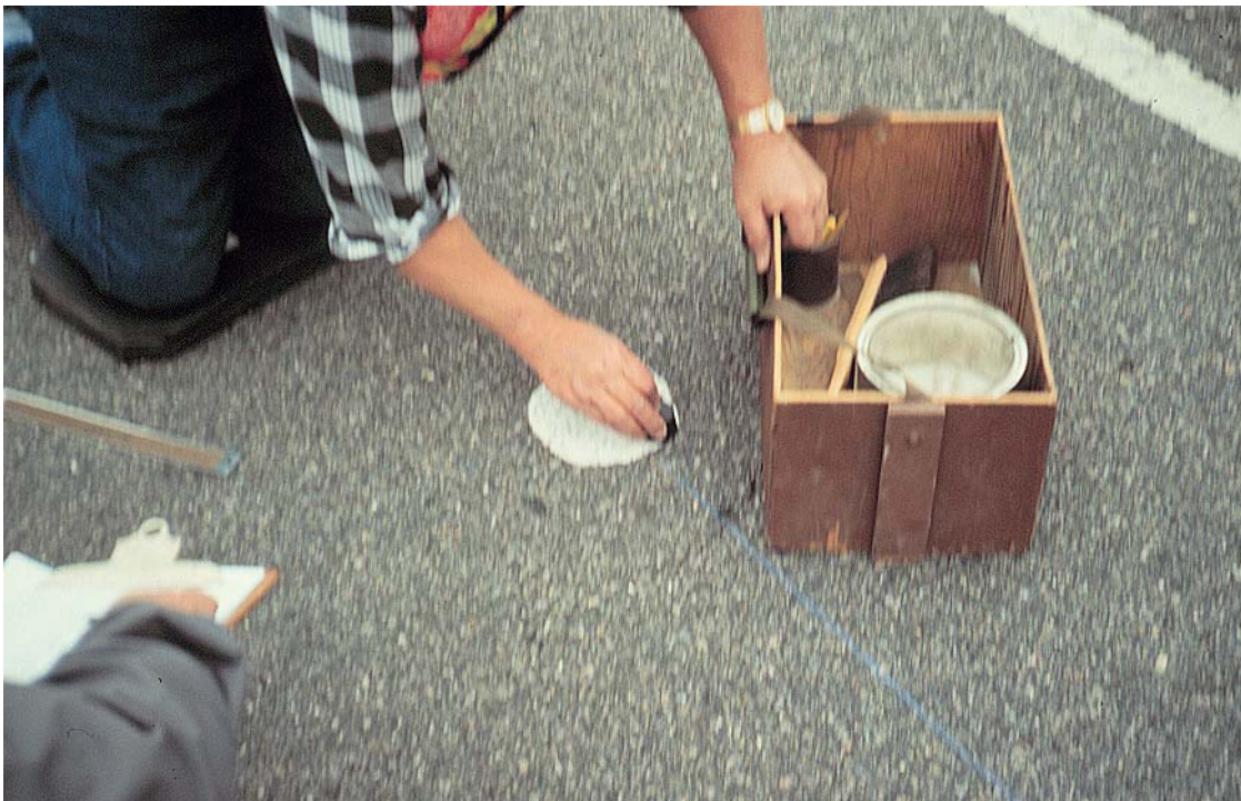
Figure 1. Volumetric Method (Sand Patch Test) (ASTM E965)
