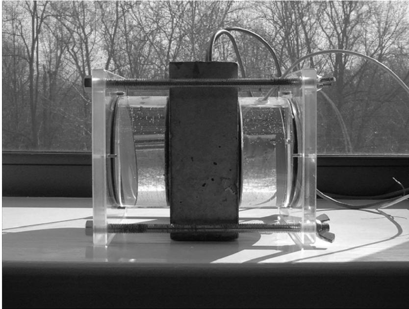
**Figure 3. Photograph of Apparatus for Electrochemical Driving of Chloride into Concrete.**
