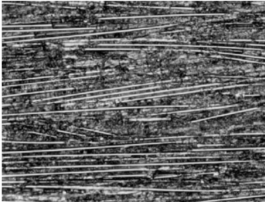
Figure 2. Optical micrograph of polished composite surface showing fiber misorientation (200x).
