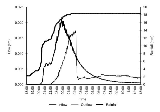
Figure 8. Typical flow and precipitation data collected at monitoring station
