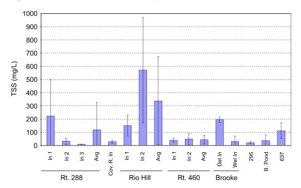
surface contributed to high levels. Figure 9 illustrates mean TSS inflow concentrations at study sites, with error bars showing one standard deviation. In general, greater variability was observed for higher mean concentrations.
