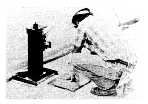
Figure 25. A template should be used to center ACI 503R pull-off device over pipe cap. A dynamometer with a capacity of at least 2,000 lbs should be hooked to the pipe cap and the loading hook and the load applied at the rate of 100 lbs every 5 sec. The dynamometer reading at rupture and the type failure, as percent concrete, bond, and overlay should be recorded.
