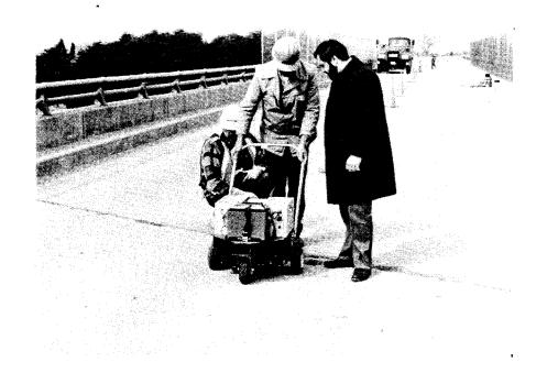
Figure 5. A delamtect can be rolled over the deck surface to produce a strip chart that can be examined to identify delaminated areas.
