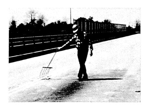
Figure 4. Several chains hanging from a pipe (chain drag) can be dragged over the deck surface to locate delaminated and very unsound concrete. The chain produces a hollow sound when it passes over delaminated concrete.
