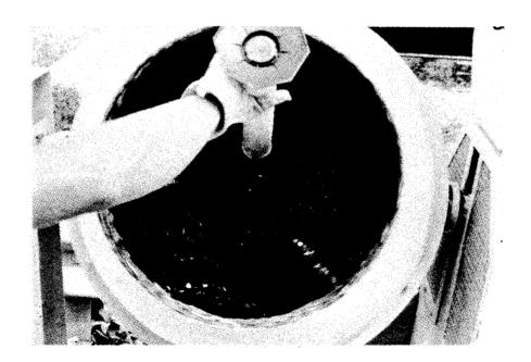
Figure 34. Methyl ethyl ketone peroxide initiator is here added to the mixer.
