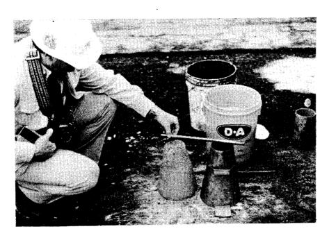
Figure 29. A slump test (ASTM C143) can provide an indication of the workability of hydraulic cement concrete. The temperature and the air content of the concrete should also be measured and recorded.
