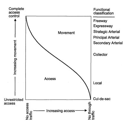
Figure 1. Relationship between highway access and mobility. Source: Koepke and Levinson, Transportation Research Board, Access Management Guidelines for Activity Centers (Report No. 348, 1992).
