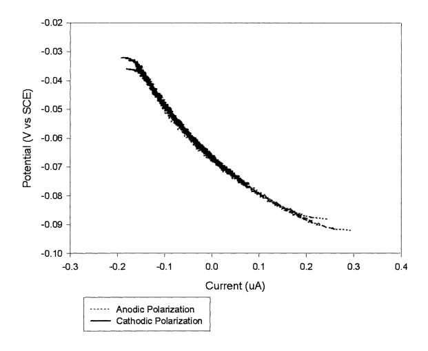
Figure 22. The micro-polarizability and hysteresis behavior of the Au-Sn, noble-passive couple in quiescent saturated calcium hydroxide. This couple exhibits limited hysteresis, returning to steady state readily.
