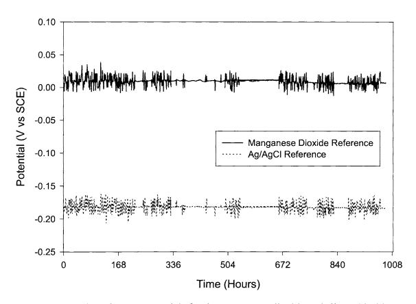
Figure 45. The reference potentials for the manganese dioxide and silver chloride commercial electrodes in concrete with chloride over 1000 hours. Both electrodes show similar, stable behavior. The standard deviations of these electrodes are caused by noise and not drift.
