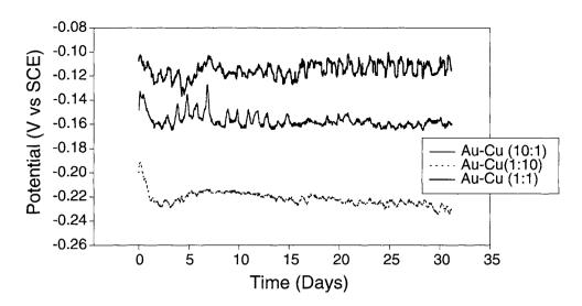
Figure 32. The open circuit potential of the Au-Cu (noble-noble) couple with cathode to anode ratios of 1:1, 1:10, and 10:1 in quiescent saturated calcium hydroxide.
