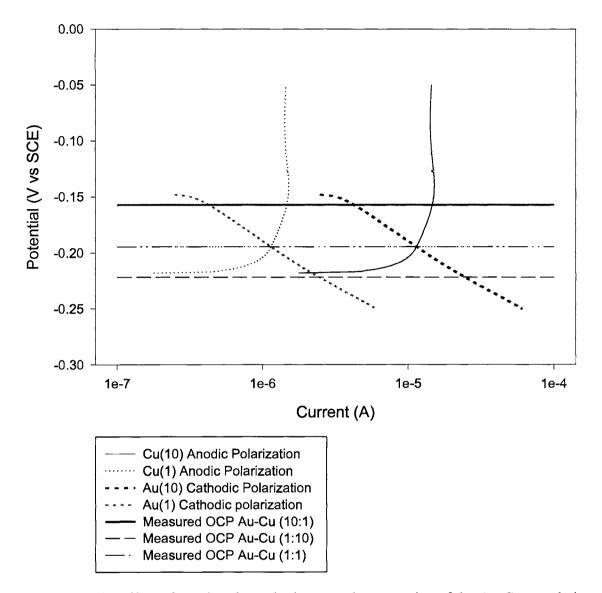
Figure 37. The effect of varying the cathode to anode area ratios of the Au-Cu couple in quiescent saturated calcium hydroxide as predicted by the mixed potential behavior of the individual couple halves after reaching steady state as a couple.
