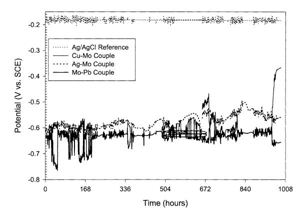
Figure 49. The potential behavior for 1000 hours in concrete with chloride of the nobleactive and active-active couples that contained molybdenum. The Ag-Mo, Cu-Mo, and Mo-Pb couples were controlled by the molybdenum in this environment. All of these couples were unstable by large noise values.
