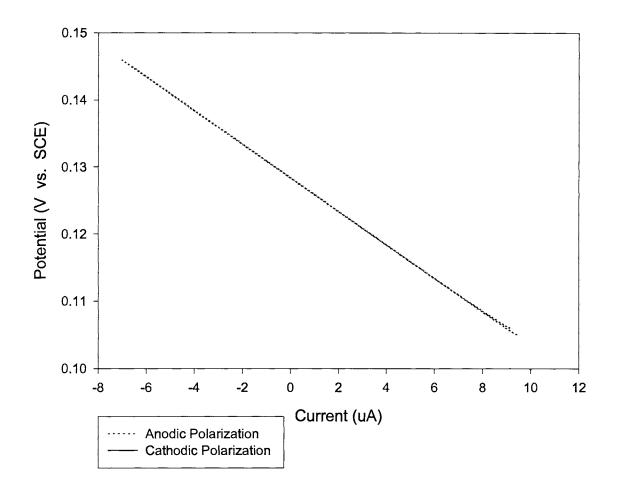
Figure 17. the micro-polarizability of true reference electrodes. The manganese dioxide reference electrode is shown.
