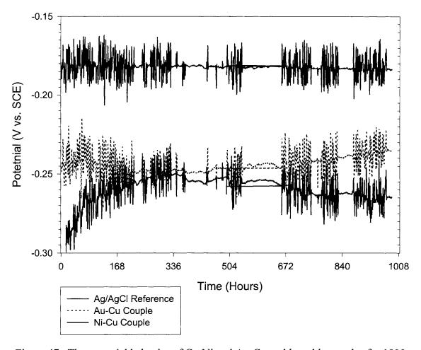
Figure 47. The potential behavior of Cu-Ni and Au-Cu, noble-noble couples for 1000 hours in concrete with chloride. The Au-Cu and Cu-Ni couples were reasonably stable in this environment. The standard deviations resulted from noise and a slight initial potential drift in the Cu-Ni couple.
