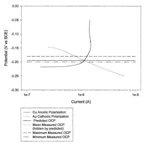
Figure 24. (a) The mixed potential behavior of the Au-Cu noble-noble couple in quiescent saturated calcium hydroxide, after reaching a steady state under coupled conditions. The predicted and measured couple potentials are shown.
