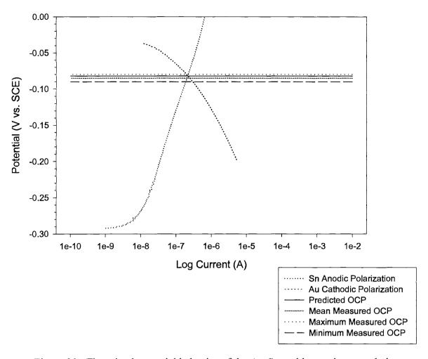
Figure 30. The mixed potential behavior of the Au-Sn, noble-passive, couple in quiescent saturated calcium hydroxide after reaching steady state under coupled conditions.
