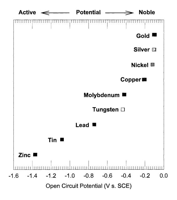
Figure 11. A galvanic series of couple components in saturated calcium hydroxide. More active metals are shown in the lower left and proceed upwards to the right in nobility.
