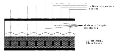
2.5 L Saturated Calcium Hydroxide Solution
