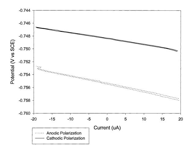
Figure 20. The micro-polarizability of the Ag-Pb, noble-active couple in quiescent saturated calcium hydroxide. The anode control of this couple provides high stability and low polarizability.
