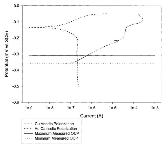
Figure 25. The mixed potential behavior of the Au-Cu couple after reaching steady state under coupled conditions in deaerated, saturated calcium hydroxide.
