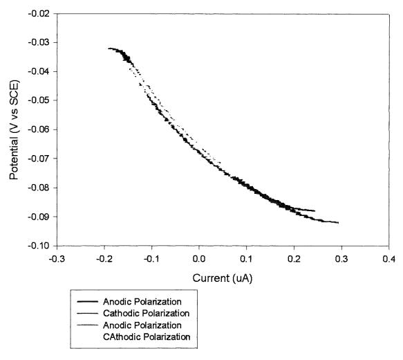
Figure 23. Micro-polarization and hystersis behavior for the Au-Sn, noble-passive couple in decreased saturated calcium hydroxide. Greater hysteresis is observed in this situation than found in quiescent solution.
