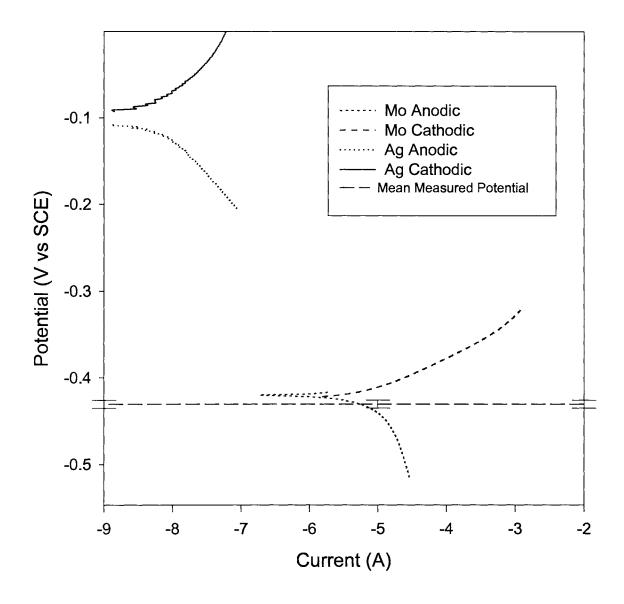
Figure 28. The separate polarization behaviors of Ag and Mo after reaching steady state under uncoupled conditions in saturated calcium hydroxide. The cathodic reaction is extrapolated to intersect the anodic reaction and determine the couple potential.
