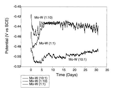
Figure 36. the effect of varying cathode to anode area ratios (1:1, 1:10, and 10:1) on the open circuit behavior of the Mo-W (active-active) couple in quiescent saturated calcium hydroxide.
