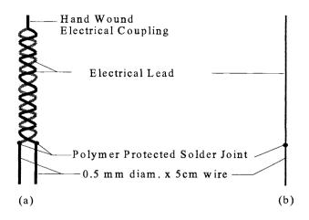
Figure 6. The form of split couple and single metal electrodes.
