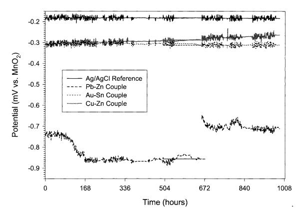
Figure 51. The potential behavior for the noble and active-passive couples in concrete with chloride for 1000 hours. The Pb-Zn couple exhibits unstable behavior by a large potential shift (similar to the lead anode couples). The Cu-Zn couple is more stable in this concrete block, but its standard deviation occurs both by slight drift and noise. The Au-Sn couple is stable, and its standard deviation occurs by noise alone.
