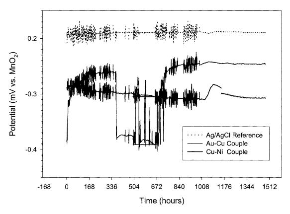
Figure 40. The potential behavior of Cu-Ni and Au-Cu, noble noble couples for 2000 hours in concrete. The Cu-Ni couple was stable, but the Au-Cu couple was unstable.
