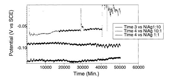
Figure 33. The open circuit potential behavior of the Ag-Ni (noble-noble) couple with cathode to anode ratios of 1:1, 1:10, and 10:1 in quiescent saturated calcium hydroxide.
