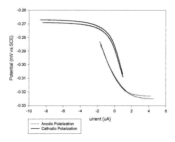
Figure 19. The micro-polarizability and hysteresis of the Au-Cu, noble-noble, couple in deaerated calcium hydroxide. The low slope seen in the polarization of this couple shows an increase in stability under deaerated conditions.
