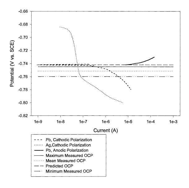
Figure 27. The polarization behavior for the split Ag-Pb, noble-noble couple, in deaerated saturated calcium hydroxide.
