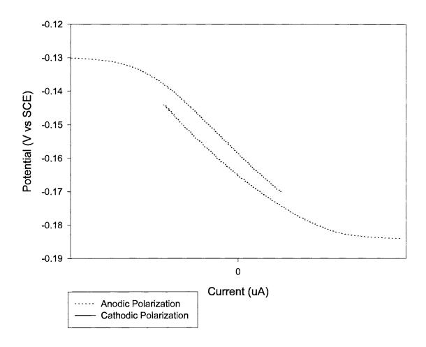
Figure 18. The micro-polarizations fo a Cu-Au, noble-noble, couple in quiescent saturated calcium hydroxide. The hysteresis in the curve shows the recovery of the couple from the polarized state back to steady state.
