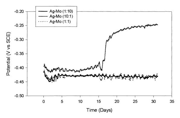
Figure 34. The effect of varying cathode to anode area ratios (1:1, 1:10, and 10:1) on the open circuit behavior of the Ag-Mo (noble-active) couple in quiescent saturated calcium hydroxide.
