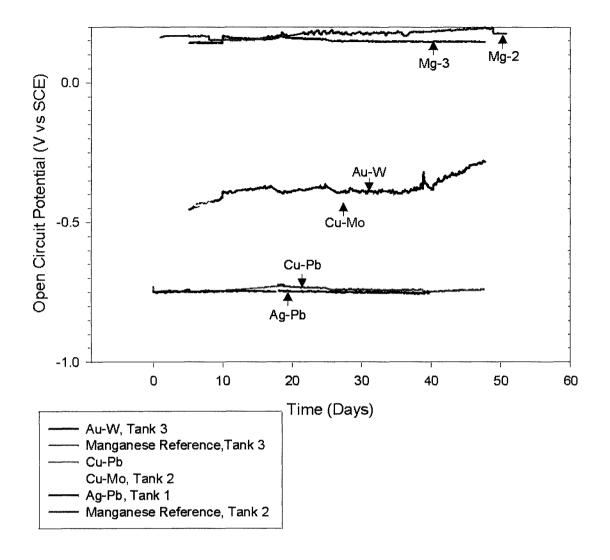
Figure 14. The open circuit behavior of noble-active couples. Successful couples have open circuit values that exhibit little drift and low standard deviations relative to the manganese dioxide reference. The unsuccessful couple has a steep drift in potential with time.
