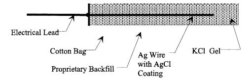
Figure 1. The structure of an embeddable silver-silver chloride electrode.
