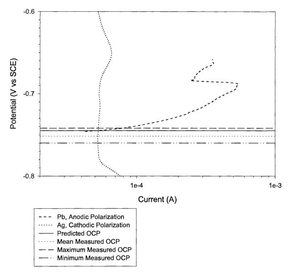
Figure 26. The polarization behavior of the anode and cathode of the Ag-Pb, nobleactive couple after reaching steady state under coupled conditions. The intersection of the anodic and cathodic currents is plotted to show the predicted couple potential along with the mean, maximum and minimum measured couple potentials.
