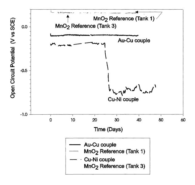
Figure 13. The open circuit behavior of successful and unsuccessful noble-noble galvanic couple electrodes. The unsuccessful electrode is marked by high noise and a large potential step. The successful electrode has low noise and as little drift as the manganese dioxide reference electrode.
