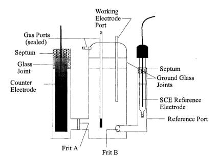
Figure 9. A schematic of the three-port electrochemical cell used in single metal electrode potentiodynamic scans.
