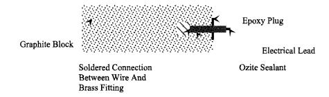
Figure 3. The structure of a graphite pseudo reference electrode.
