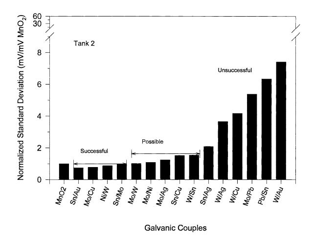
Figure 12 (b). Normalized standard deviations for Tank 2.
