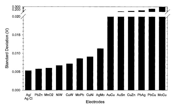
Figure 39. The standard deviations of the commercial and galvanic couple reference electrodes for 2000 hours in concrete.
