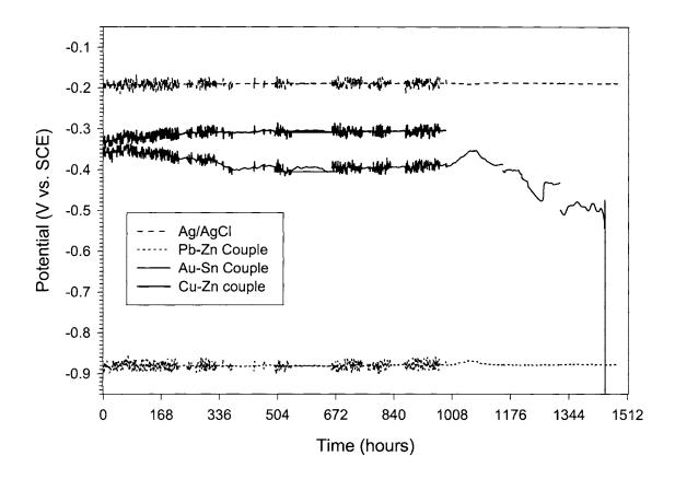
Figure 44. The potential behavior for the noble and active-passive couples in concrete for 2000 hours. The Pb-Zn couple exhibits stable behavior. The Au-Sn and Cu-Zn couples both lost stability in large potential shifts.
