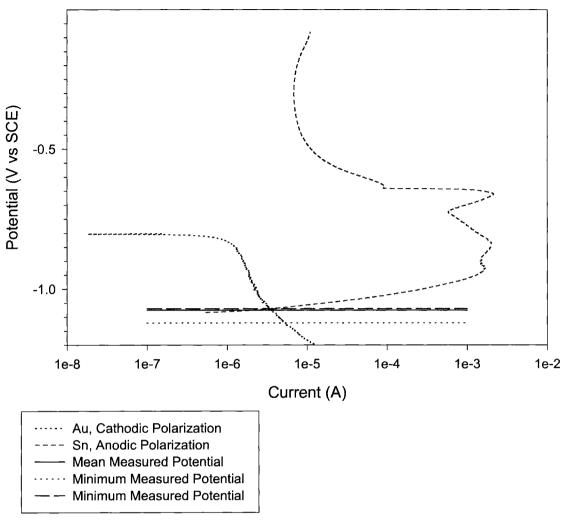
Figure 31. The mixed potential behavior of the Au-Sn, noble-passive, couple in deaerated saturated calcium hydroxide after reaching steady state under coupled conditions.
