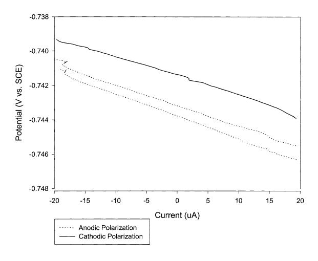
Figure 21. The micro-polarizability and hysteresis behavior of the Ag-Pb, noble-active couple in deaerated, saturated calcium hydroxide solution. This couple has a low polarizability in deaerated solution.
