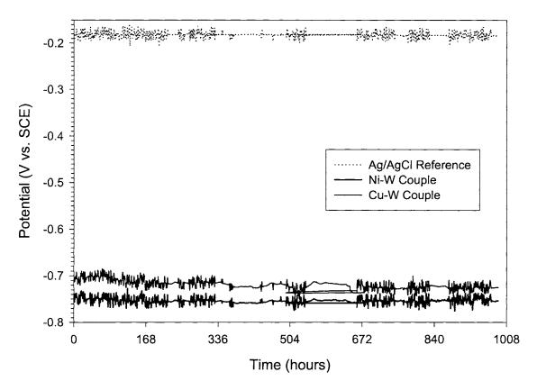
Figure 50. The potential behavior for 1000 hours in concrete with chloride of the nobleactive couples that contained tungsten. The Ni-W and Cu-W couples both exhibit stable potentials in concrete. Their standard deviations occur as noise.
