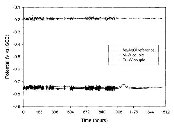
Figure 43. The potential behavior for 2000 hours in concrete of the noble-active couples that contained tungsten. The Ni-W and Cu-W couples both exhibit stable potentials in concrete. Their standard deviations occur as noise.
