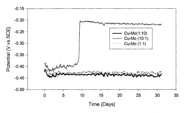
Figure 35. the effect of varying cathode to anode area ratios (1:1, 1:10, and 10:1) on the open circuit behavior of the Cu-Mo (noble-active) couple in quiescent saturated calcium hydroxide.
