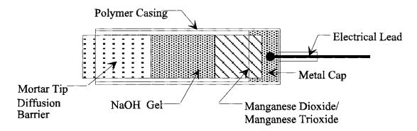
Figure 2. The structure of a MnO<sub>2</sub>/Mn<sub>2</sub>O<sub>3</sub> embeddable reference electrode.
