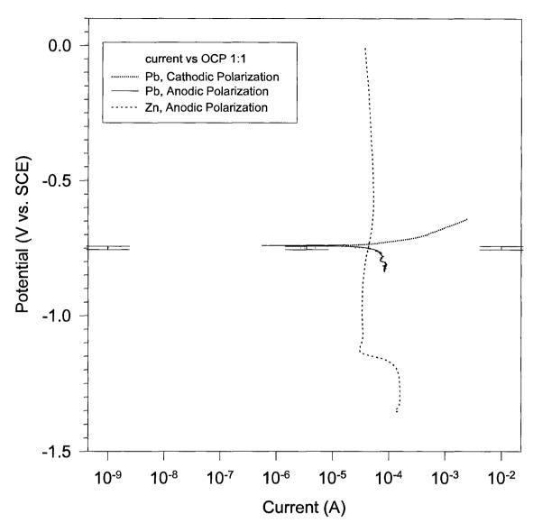
Figure 29. The single metal polarization behavior of Pb and Zn, showing the mixed potential behavior of the Pb-Zn (active-Passive) couple. The couple potential falls near the open circuit potential of Pb.
