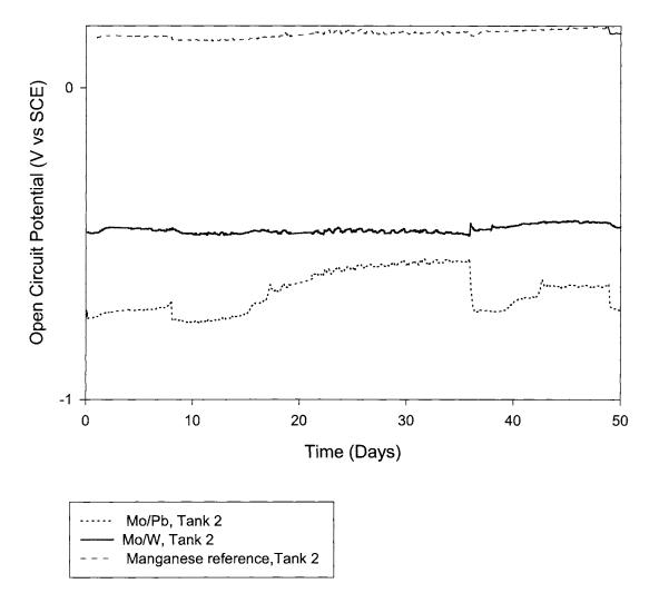
Figure 16. The stability behavior of active-active galvanic couples in saturated calcium hydroxide shows that stable couples (Mo-W) have steady open circuit potentials like the manganese dioxide reference electrode, but unstable electrodes (Mo-Pb) have large potential shifts.
