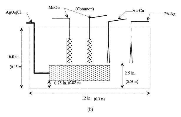
Figure 10. the electrode setup within the concrete blocks: (a) the top view of the electrode, and (b) a cut-away view of the center row of electrodes.
