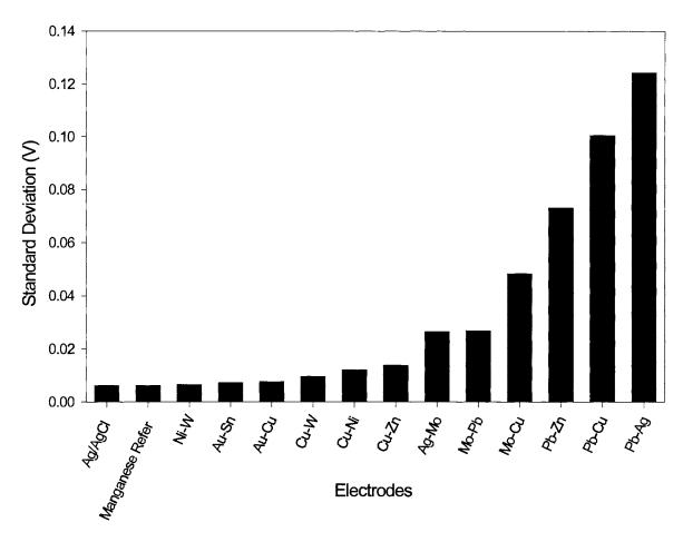
Figure 46. The standard deviations of the commercial and galvanic couple reference electrodes for 1000 hours in a chloride, concrete environment.
