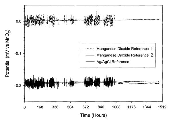
Figure 38. The reference potentials for the manganese dioxide and silver chloride commercial electrodes in concrete over 2000 hours. The stability of the Ag/AgCl electrode is plotted as determined against both manganese electrodes. All three electrodes show similar, stable behavior. The standard deviations of these electrodes are caused by noise and drift.
