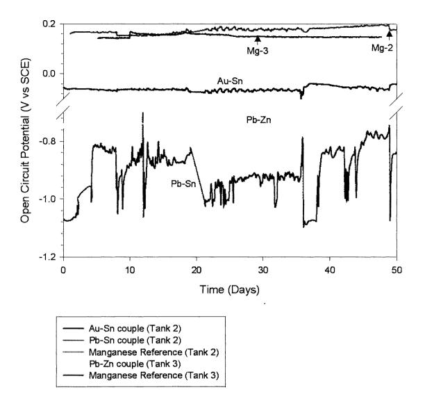
Figure 15. The stability behavior of noble/active galvanic couples in saturated calcium hydroxide. The open circuit behavior of the successful couples has extremely low noise (standard deviation) compared to the large variations seen in the unsuccessful Pb-Sn couple.
