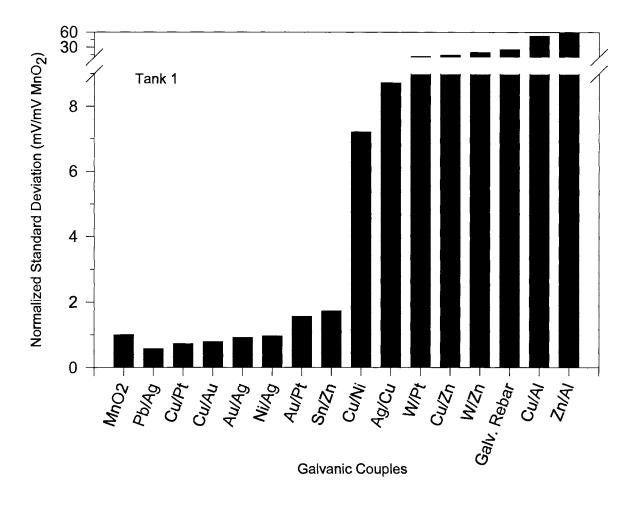
Figure 12. The normalized standard deviations for electrodes in (a) Tank 1, (b) Tank 2, and (c) Tank 3, range from less than 1 (better than the associated MnO<sub>2</sub> electrode) to greater than 60 mV/mV. The ranges of successful, unsuccessful, and promising electrodes can be obtained from these standard deviations.
