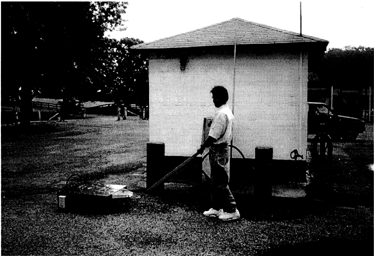
Figure 4. Scanning a location by towing the antenna over it.
