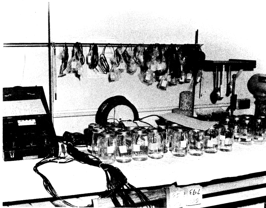
Figure 4. Calibration of moisture gages in distilled water.
