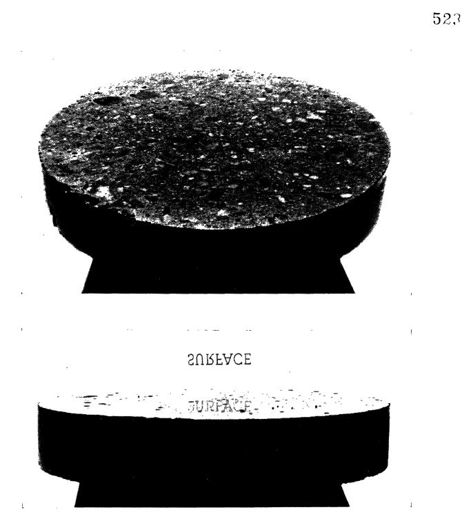
Figure 3. These photographs of the same well-prepared surface illustrate the quality of the surfaces required for microscopical examination and analyses. A. The surface viewed in ordinary illumination. B. The surface viewed at a very low angle toward a source of illumination. The quality of the reflection of a distant object (here, the quality of the reflection of the reversed word "SURFACE" on the screen) indicates the flatness of the lapped surface.
