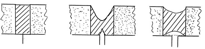
Figure 4. Sealant behavior with and without a bond breaker at the lower seal-concrete interface. After Schultz. (5)
