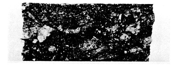
Figure 11. Typical stripping in coarse aggregate.
