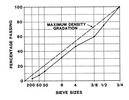
Figure 3. Experimental mix gradation plotted in relation to maximum density gradation.
