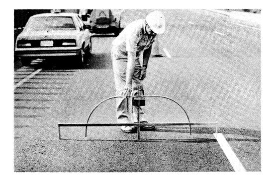
Figure 9. Six-foot bow used to measure ruts.
