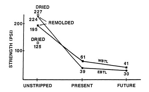
Figure 5. Deterioration curves for I-2 mix on I-64.
