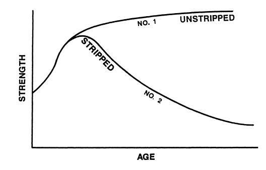
Figure 1. Strength vs. age of pavement.
