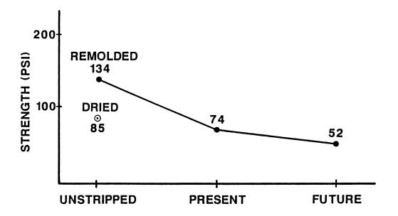
Figure 7. Deterioration curve for Greenwood Drive.
