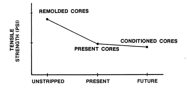
Figure A-1. Typical deterioration curve.
