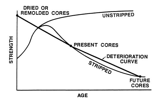
Figure 2c. Deterioration curve.
