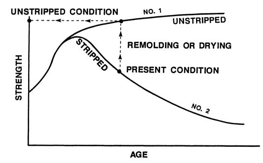
Figure 2a. Development of deterioration curve (present and unstripped conditions).
