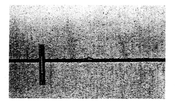
Figure 11. Cohesive and some adhesive loss for the type C sealant.
