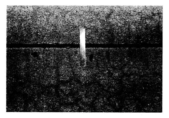
Figure 12. Overlapping failure for type C sealant.
