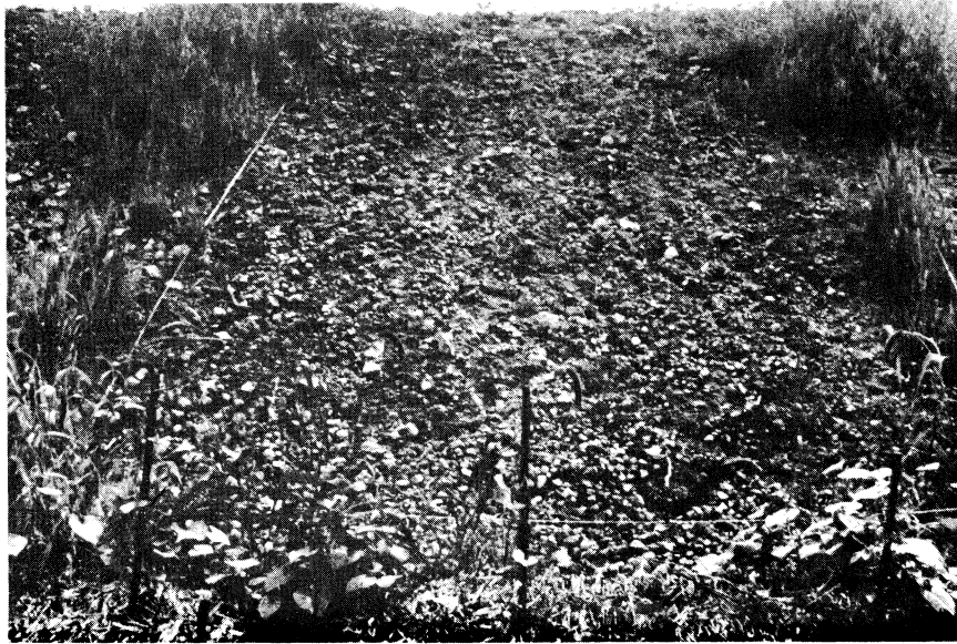
Plate 3. Dow NC-1556.2L — 3 months. Page County — Rating No. 6. Sheet erosion in middle of plot.
