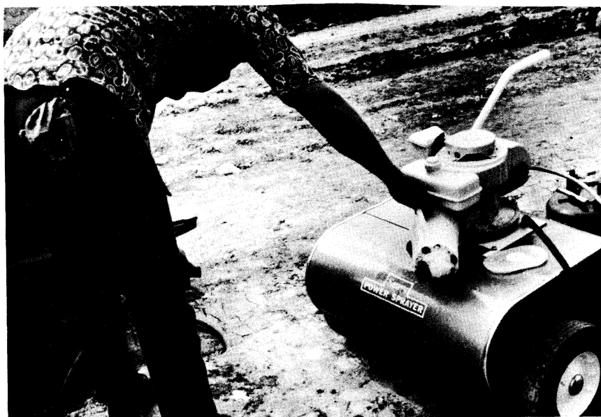
Figure 3. 3 hp. , 20-gallon sprayer used.
