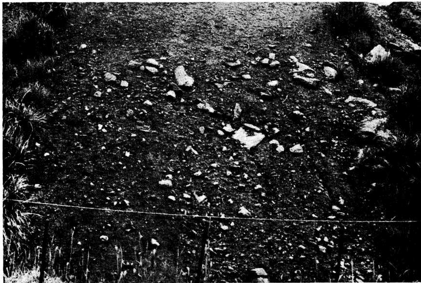
Plate 8. Aerospray 70 — 5 1/2 months. Greene County — Rating No. 1. Rills on right side are approximately 1" deep.
