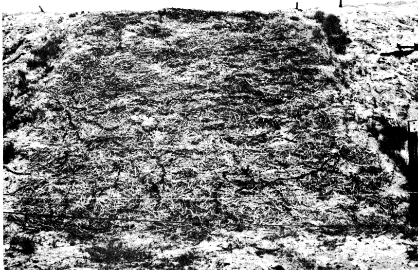
Plate 1. Conventional method used at all sites. 7 months — rating No. 1. This plot was treated at the rate of 2 tons of straw per acre tacked with 250 gallons of asphalt emulsion per acre.
