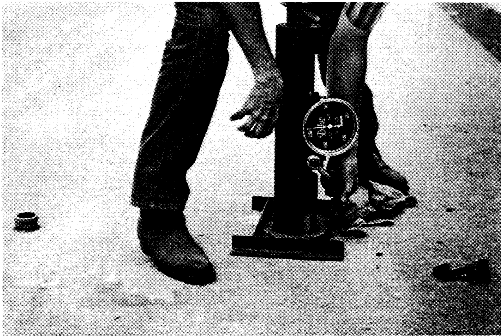
Figure 3. Apparatus used for ACI 503R surface adhesion test.
