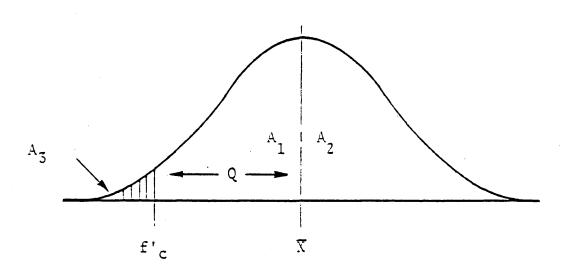
Figure 1. Significant parameters for statistical evaluation of concrete quality.
