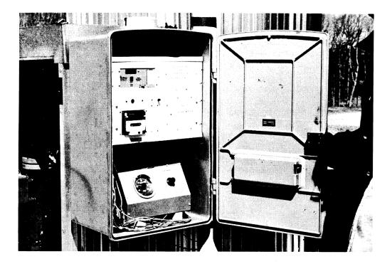
Figure 6. View of the monitoring and data recording equipment (top); flow meter (bottom).
