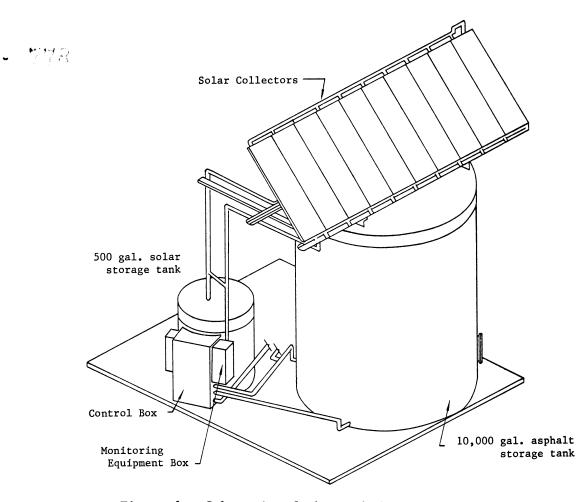
Figure 1. Schematic of the asphalt storage tank and solar heating system.
