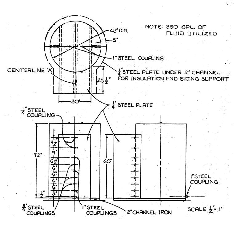
Figure A-2. Details of 500 gal. solar storage tank.
