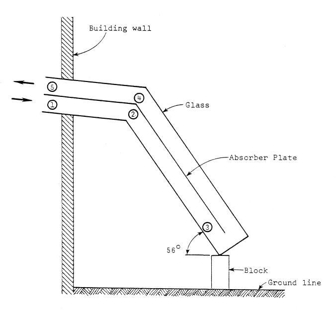
Figure 8. Points in homemade solar heater at which air temperature measurement were made.
