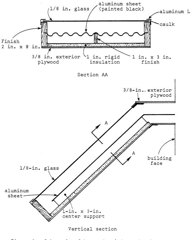
Figure 6. Schematic of homemade window solar heaters. (Courtesy of W. B. Coburn.)
