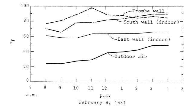
February 11. Thermal performance of the Trombe wall at Yancey Mill. (Data provided courtesy of W. B. Coburn.)
