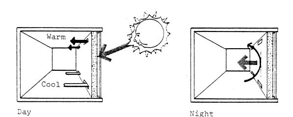
Figure 3. A Trombe wall with ventilation.
