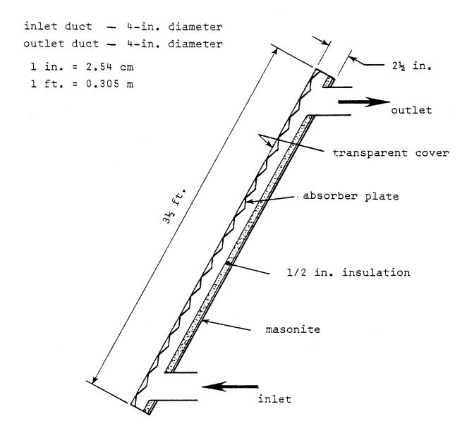
Figure 2. Cross section of creative alternative Model 2010 solar air collector.
